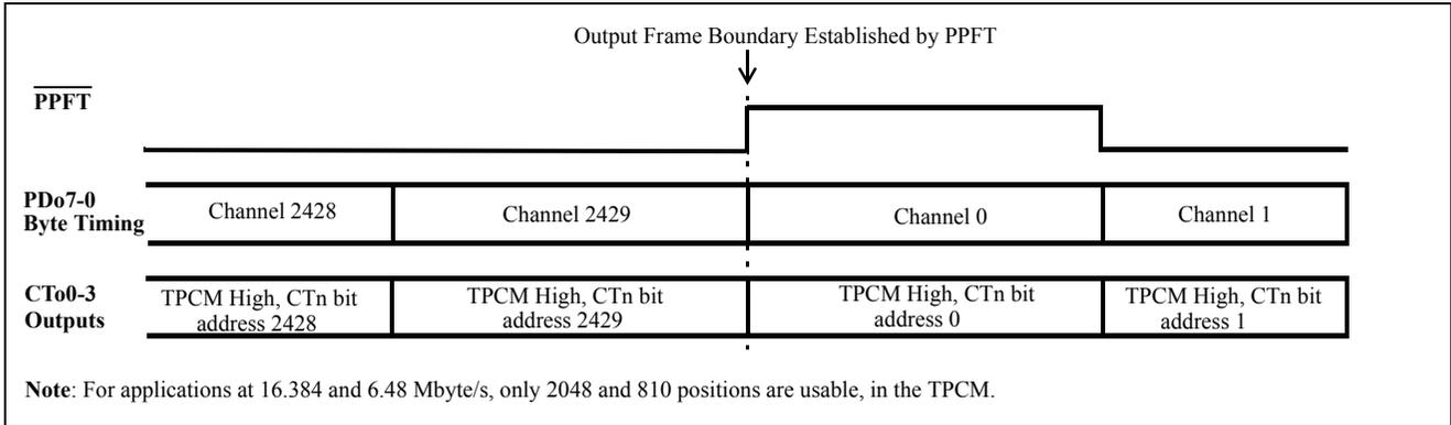
Figure 9 - Parallel Port Control Outputs, CT0-3
