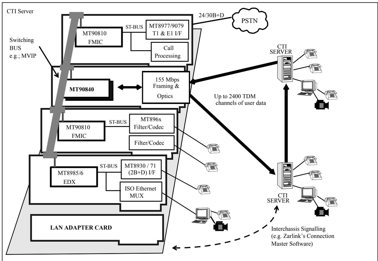
Figure 16 - CTI Distributed Architecture Implemented with the MT90840
