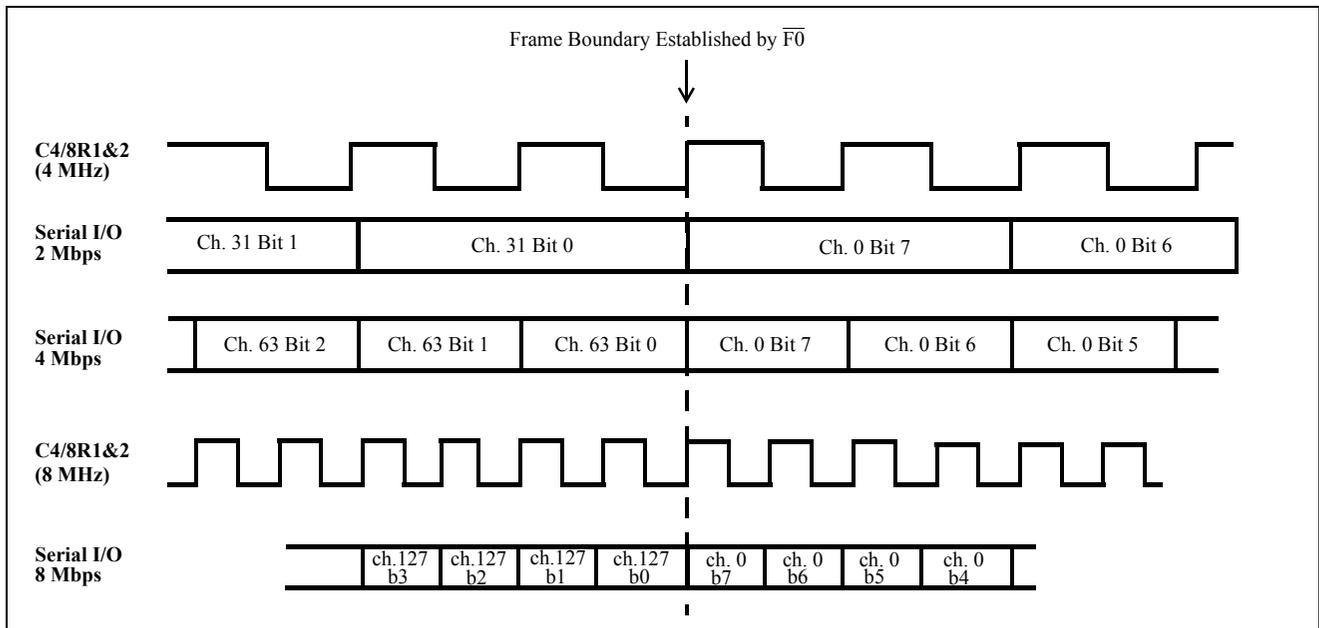
Figure 3 - Serial Port Interface Functional Timing
