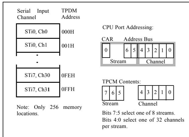
Figure 11a - 2.048 Mbps Balanced Mode TPDM Addressing
