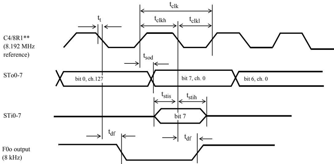
Frame Sync with Negative Polarity (SPFP = 0)
