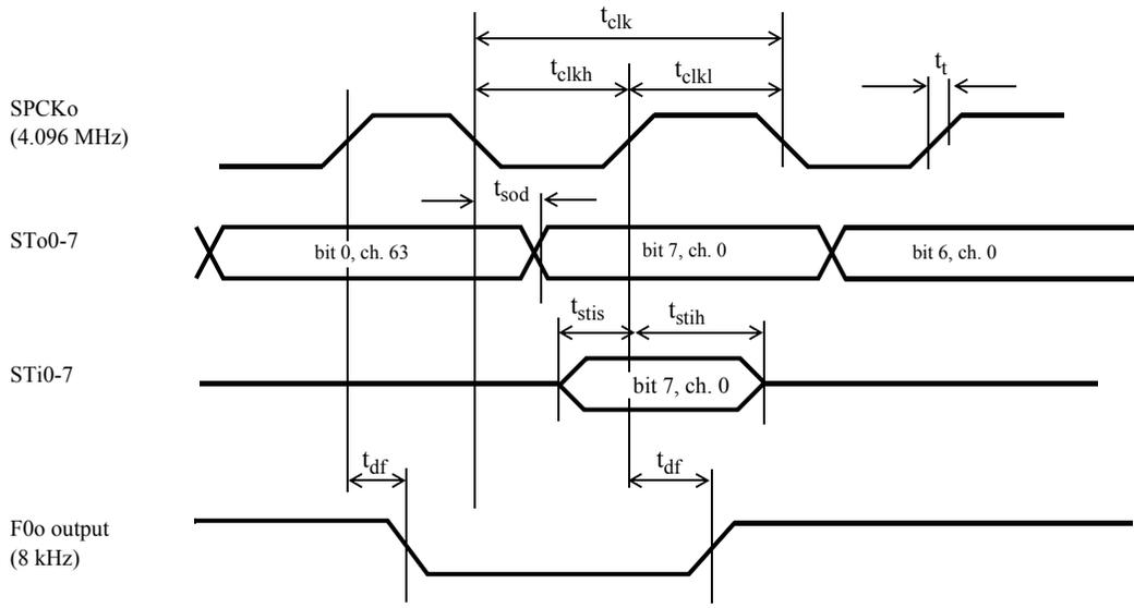
F0 Frame Sync with Negative Polarity (SPFP = 0)
