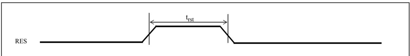
Figure 35 - RESET Timing
