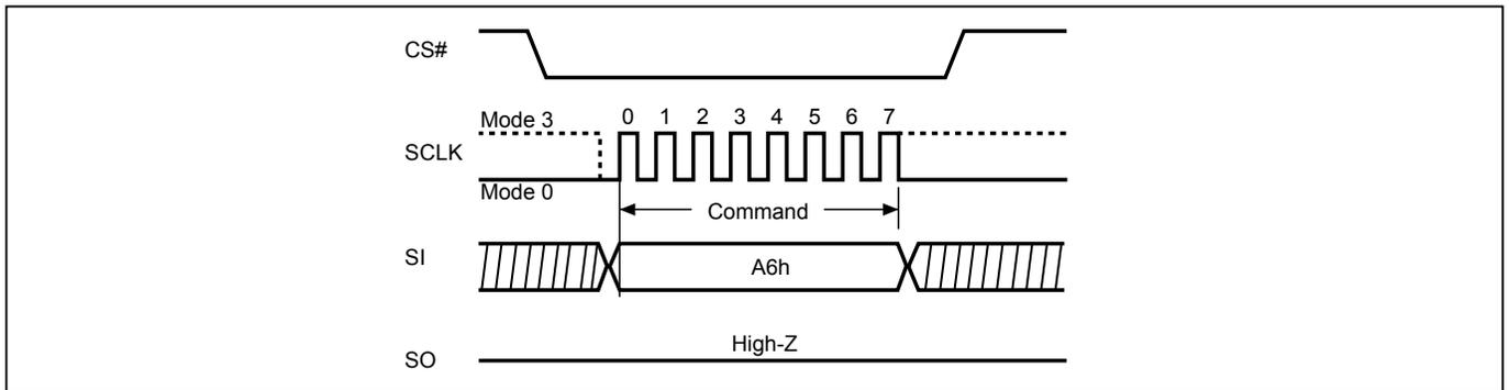
**Figure 102. Read SPB Lock Register (RDSPBLK) Sequence**
