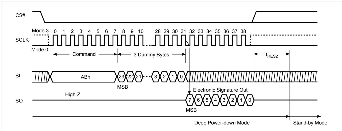
**Figure 21. Read Electronic Signature (RES) Sequence (QPI Mode)**
