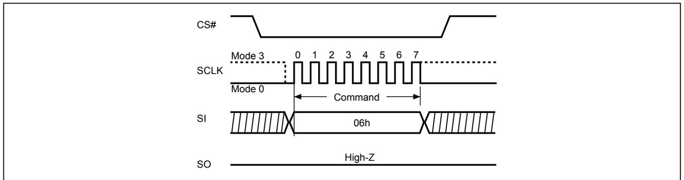
**Figure 14. Write Enable (WREN) Sequence (QPI Mode)**
