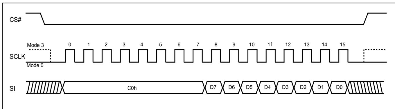
**Figure 74. Burst Read (QPI Mode)**
