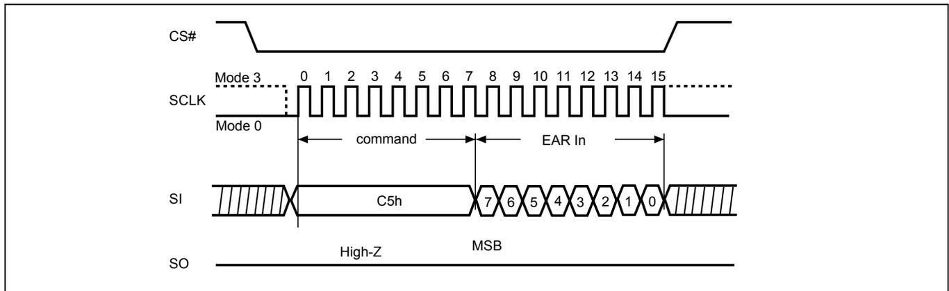
**Figure 7. Write EAR Register (WREAR) Sequence (QPI Mode)**
