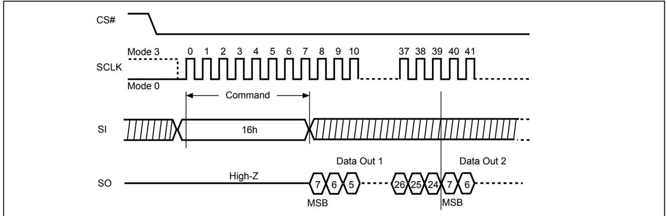
**Figure 78. Write Fast Boot Register (WRFBR) Sequence**
