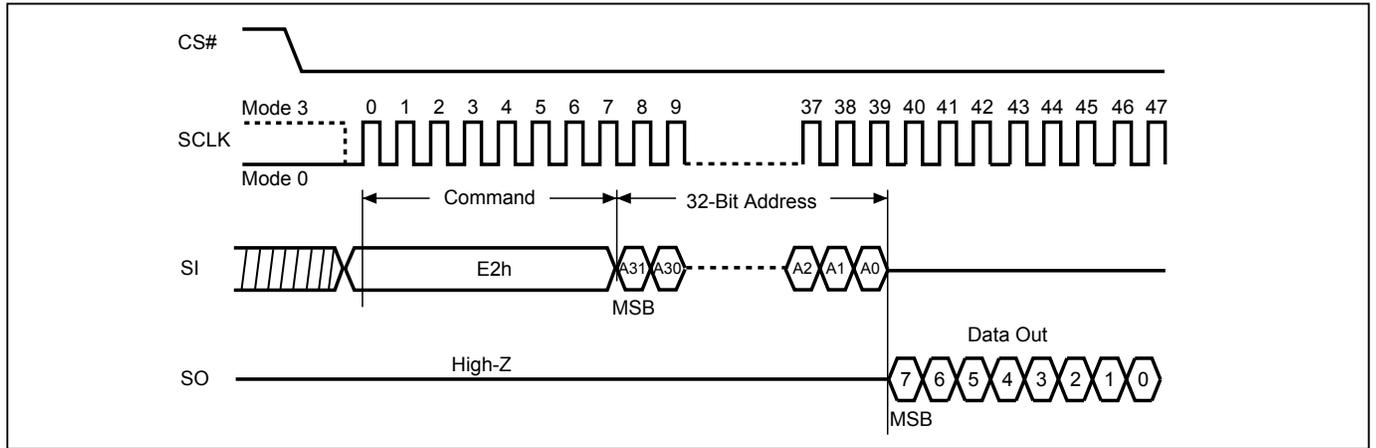
**Figure 104. SPB Erase (ESSPB) Sequence**
