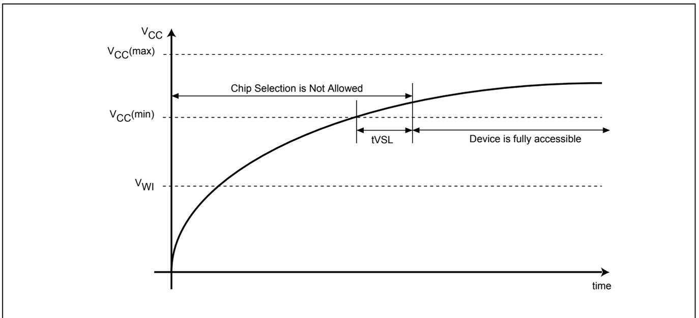
**Figure 127. Power Up/Down and Voltage Drop**
