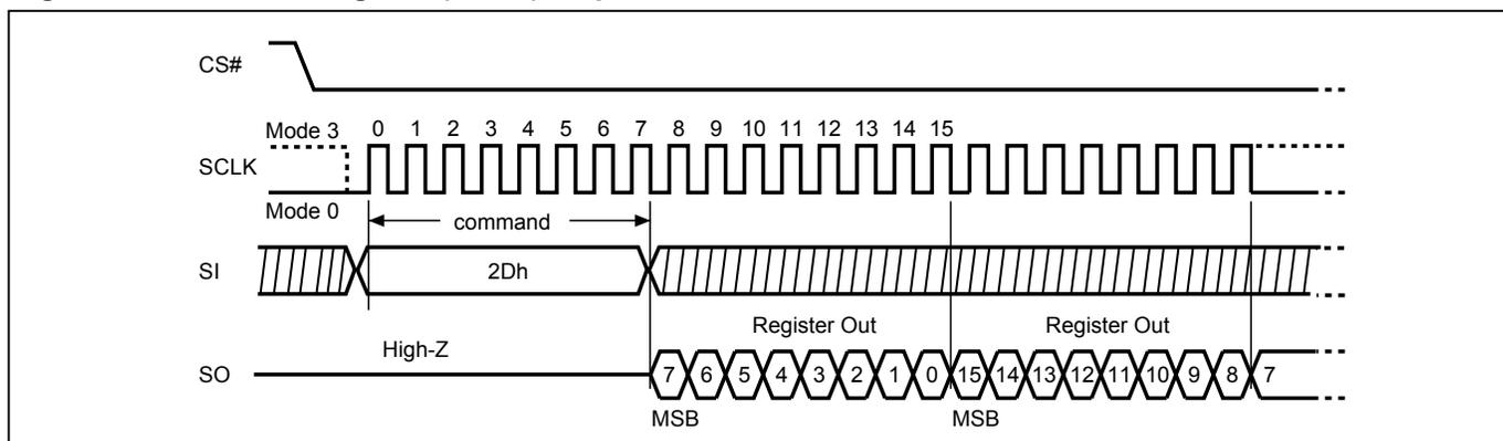
**Figure 100. Write Lock Register (WRLR) Sequence (SPI Mode)**
