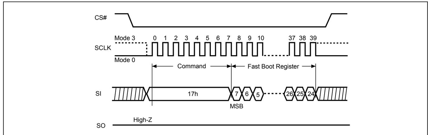
**Figure 79. Erase Fast Boot Register (ESFBR) Sequence**
