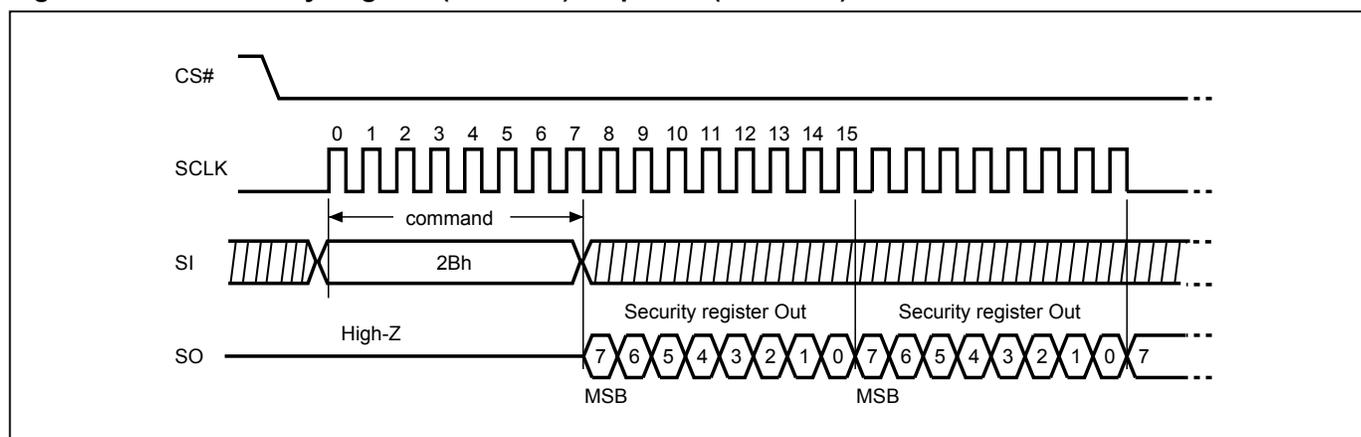
**Figure 94. Read Security Register (RDSCUR) Sequence (QPI Mode)**
