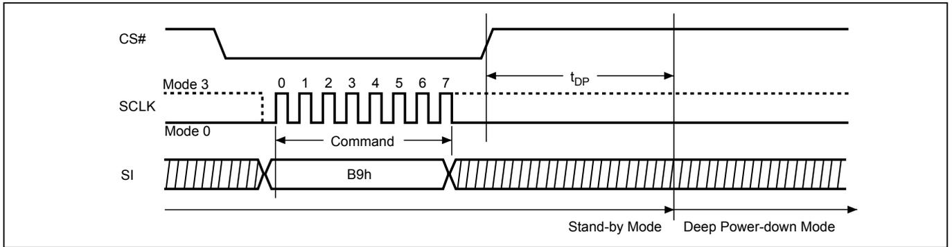
**Figure 92. Deep Power-down (DP) Sequence (QPI Mode)**
