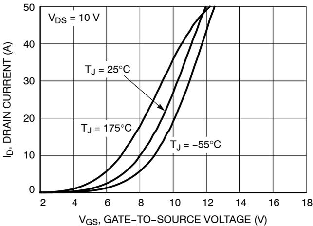
Figure 5. Transfer Characteristics
