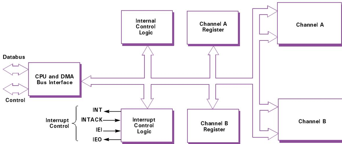
The ESCC has many improvements that significantly reduce CPU overhead. The addition of a 4-byte transmit FIFO and an 8-byte receive FIFO significantly reduces the overhead required to provide data to the transmitters, and to get data from the receivers.
