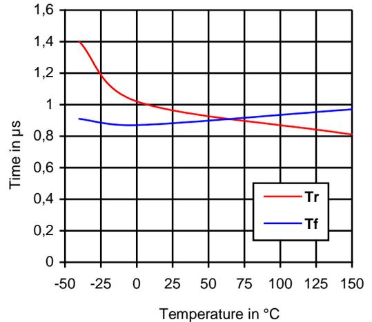
**Figure 12: Rise and fall time vs. temperature**
