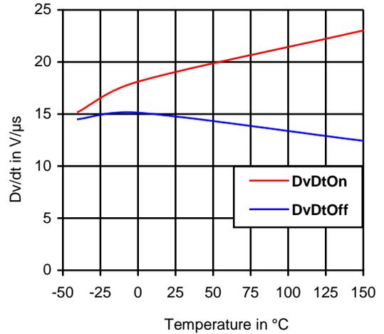
**Figure 14: Dv/dt on & off vs. temperature**
