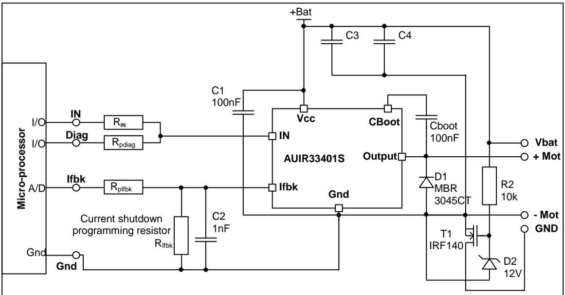
**Figure 1: Recommended schematic**
