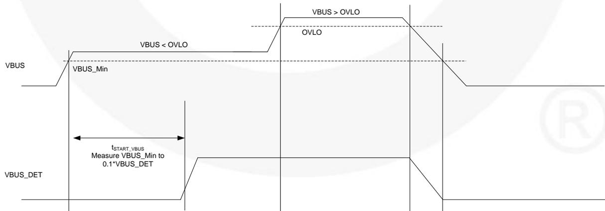
**Figure 7. Always ON V<sub>BUS\_DET</sub> Operation (ONB=HIGH)**
