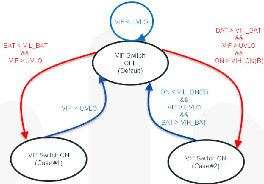
Figure 11. V<sub>IF</sub> Turn-On Qualification State Diagram
