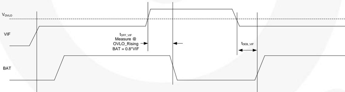
Figure 10. Timing for  $V_{IF}$  OVLO Operation (ON=Don't Care)
