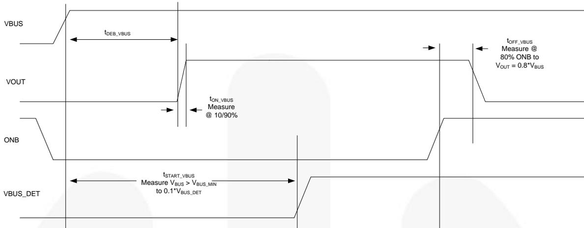
**Figure 5. Timing for V<sub>BUS</sub> Power Up/Down and Normal Operation**
