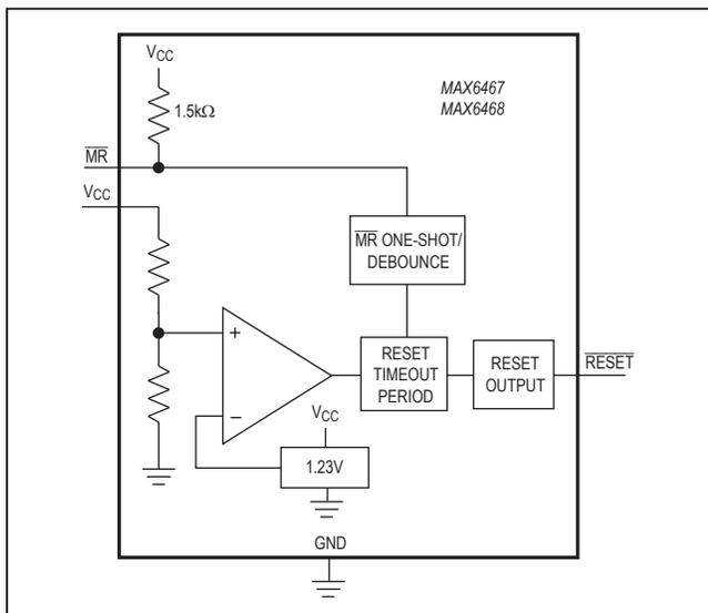
Figure 2. Functional Diagram
