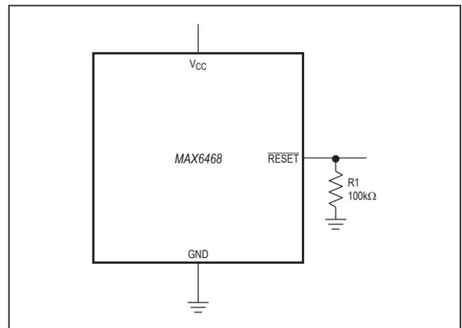
Figure 3. RESET Valid to V<sub>CC</sub> = 0V
