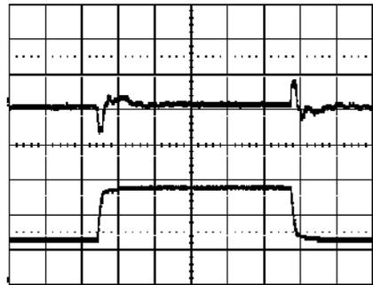
Output voltage response to load current step-
