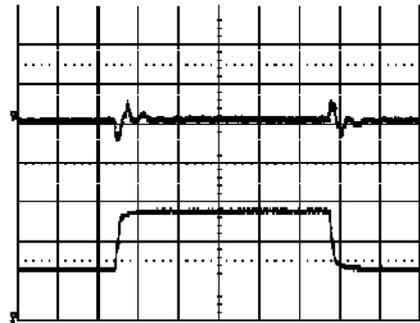
Output voltage response to load current step-
