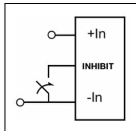
The products are equipped with a Inhibit control function referenced to the primary negative input connection (- In), positive logic. The INHIBIT function allows the regulator to be turned on/off by an external device like a semiconductor or mechanical switch.
