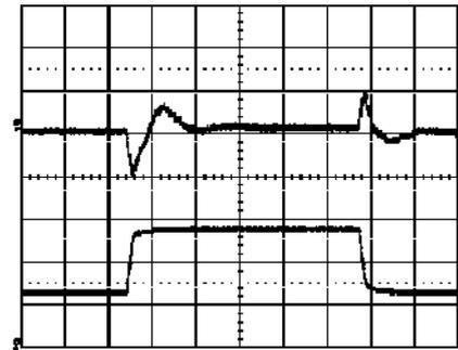
Output voltage response to load current step-
