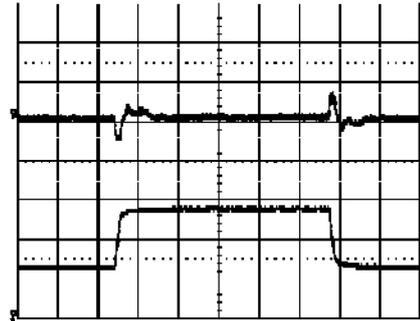
Output voltage response to load current step-
