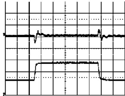
Output voltage response to load current step-
