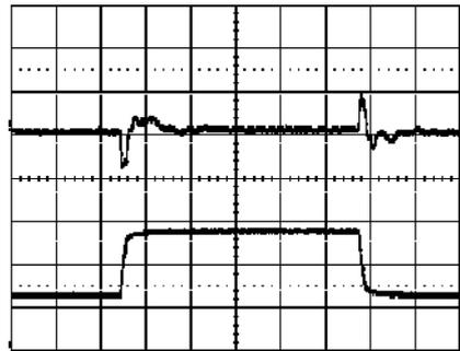
Output voltage response to load current step-
