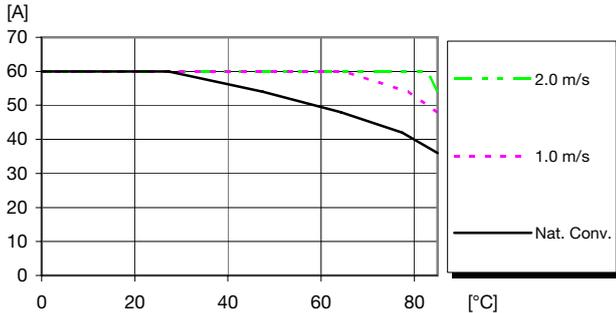
Available load current vs. ambient air temperature and airflow at  $V_I = 3.3 V, V_{OUT} = 2.0 V$ . See Thermal Consideration section.
