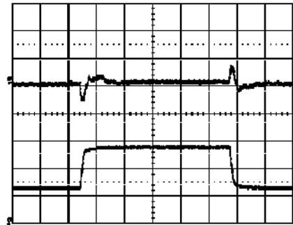
Output voltage response to load current step-
