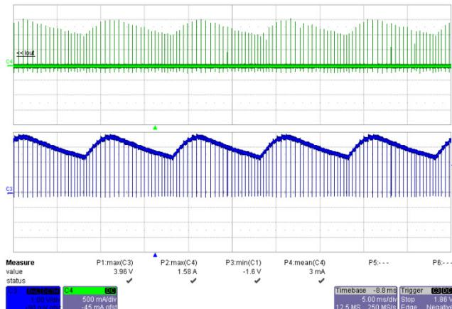
**Figure 41 – 265 VAC, 50 Hz Output Short Condition.**
