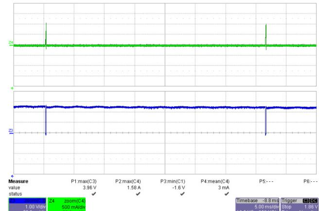
**Figure 42 – 265 VAC, 50 Hz Output Short Condition.**
