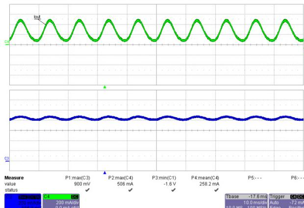
**Figure 17 – 195 VAC, 50 Hz Full Load.**
