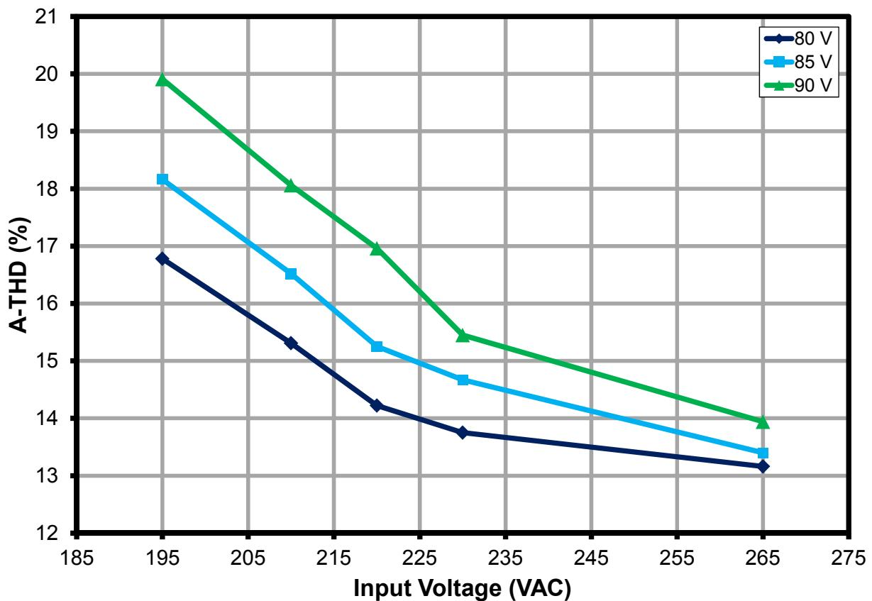
Figure 7 – A-THD vs. Line and Load.
