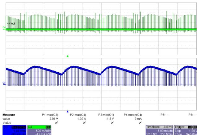
**Figure 39 – 195 VAC, 50 Hz Output Short Condition.**
