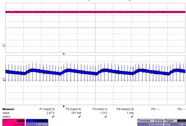
Figure 43 – 195 VAC, 50 Hz No-Load Characteristic.
