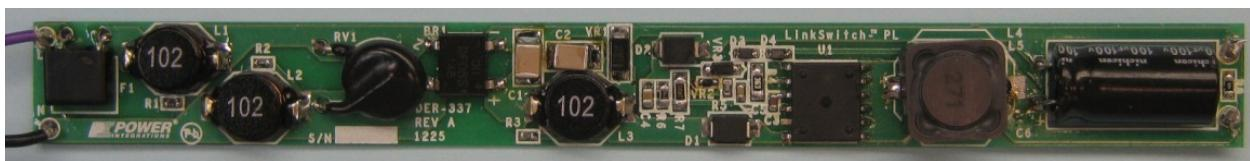
**Figure 1** – Populated Circuit Board (158 mm x 16 mm).
