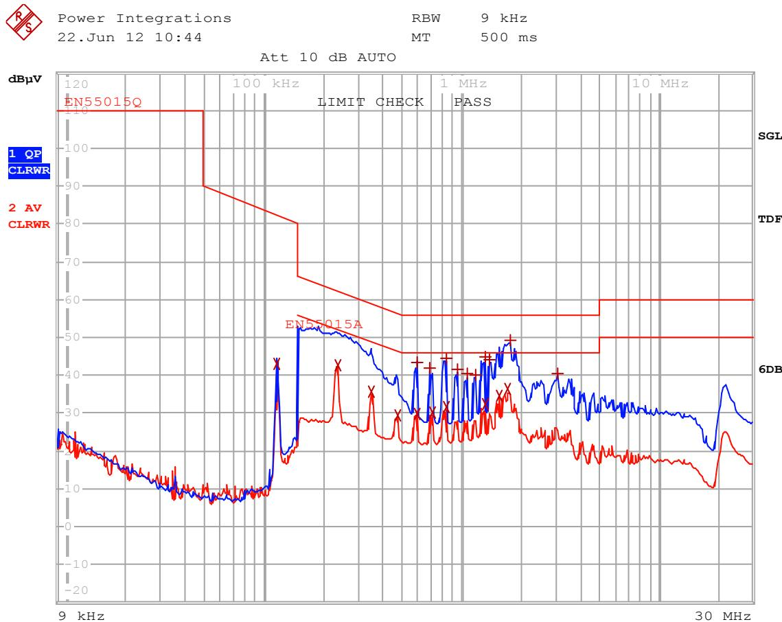
**Figure 45 –** Conducted EMI 85 V / 240 mA Load, 230 VAC, 60 Hz, and EN55015 Limits.
