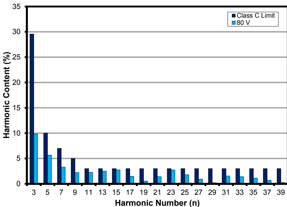
**Figure 8 – 80 V Output. Input Current Harmonics at 230 VAC, 50 Hz.**
