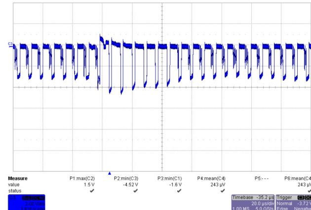
**Figure 48 –** 230 VAC, 50 Hz 2.5 kV Ring Test.
