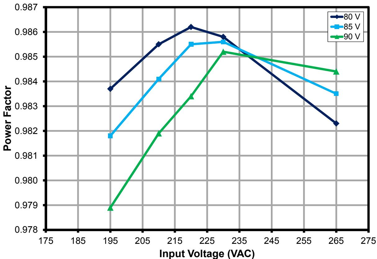
Figure 6 – Power Factor vs. Line and Load.
