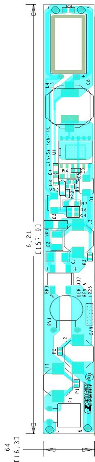
Figure 3 – Top Side (PCB Dimension: 158 mm x 16 mm).
