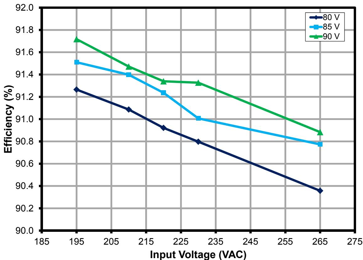
Figure 4 – Efficiency vs. Line and Load
