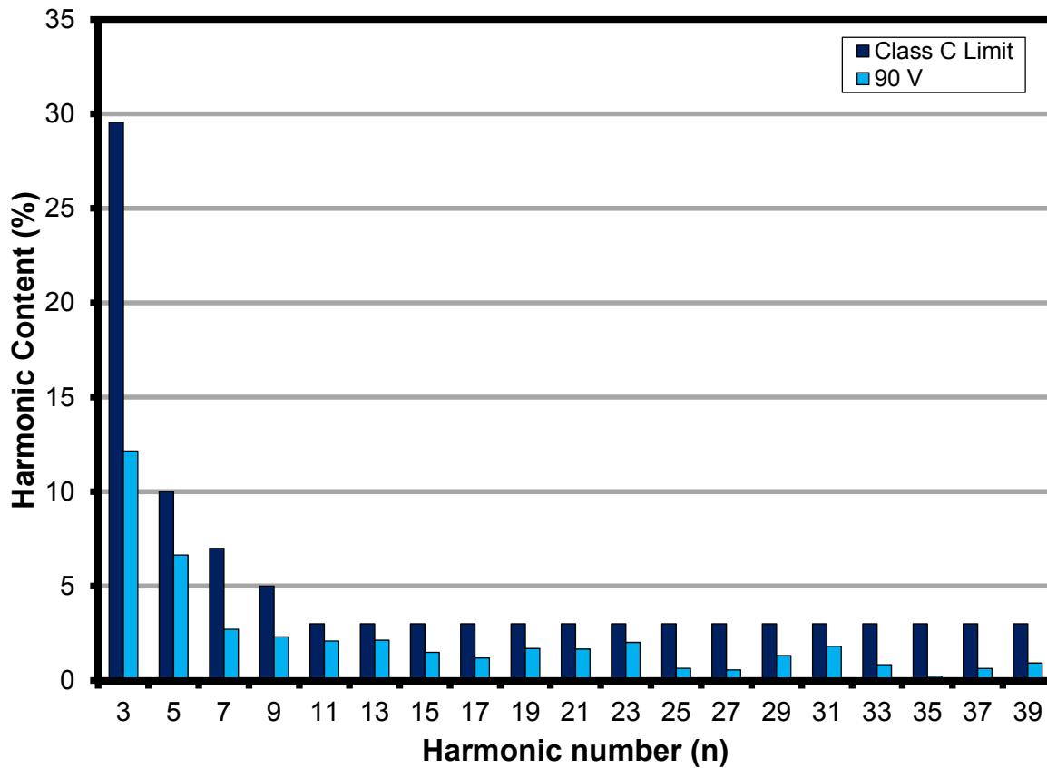
**Figure 10 – 90 V Output. Input Current Harmonics at 230 VAC, 50 Hz.**
