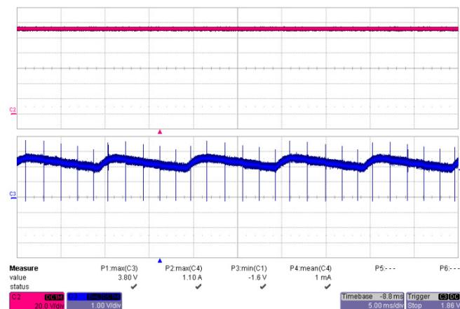
Figure 44 – 265 VAC, 50 Hz No-Load Characteristic.
