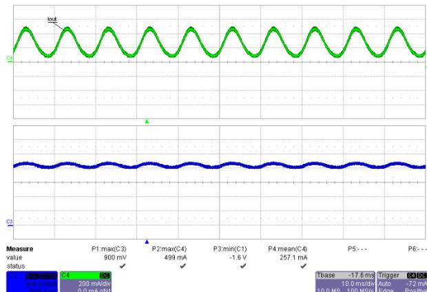
**Figure 19 – 230 VAC, 50 Hz Full Load.**
