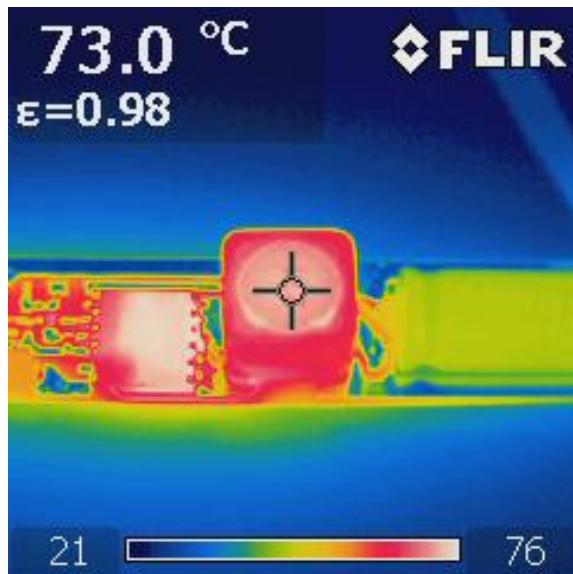
Figure 11– Output Inductor: 73 °C.
