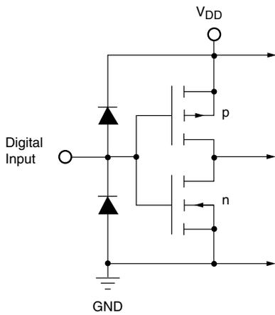
Figure 1. Equivalent Digital Input Circuit
