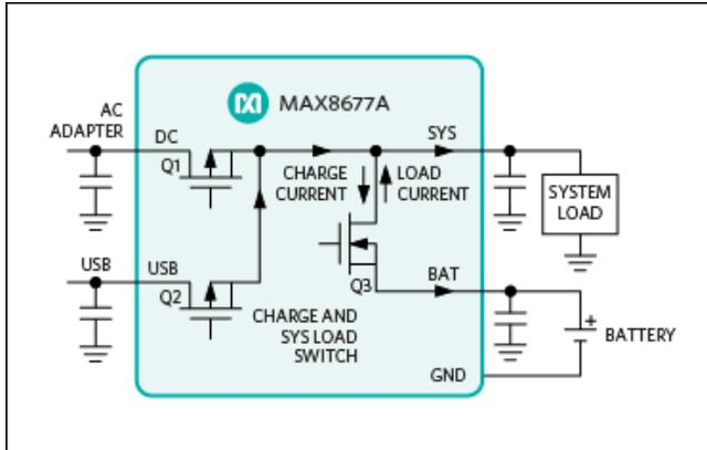
Figure 3. The Smart Power Selector technology splits the charge and load currents according to the demand.
