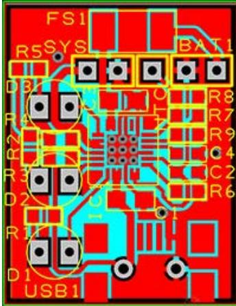
Figure 6. The PCB designed for this charger has been kept as small as possible to make it easier to build it into existing equipment.
