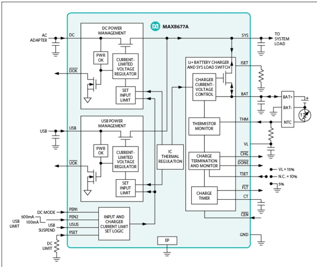
Figure 2. Block diagram of the internal circuit of the MAX8677A.
