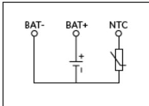
Figure 5. Most lithium-ion batteries with three connections have an internal NTC thermistor connected as shown.
