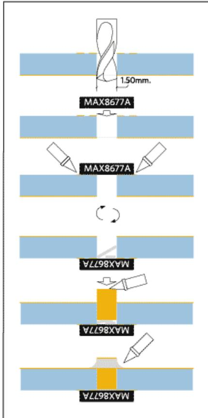
Figure 7. Steps in mounting the MAX8677A through hand-soldering a single hole.
