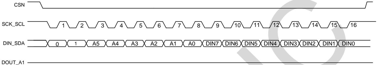
Figure 17. SPI Register Write Cycle - Single
