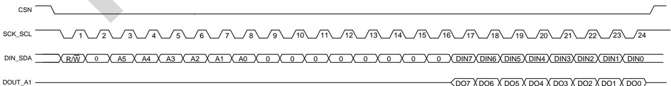
Figure 16. General SPI Protocol, 2-Byte Address (legacy)
