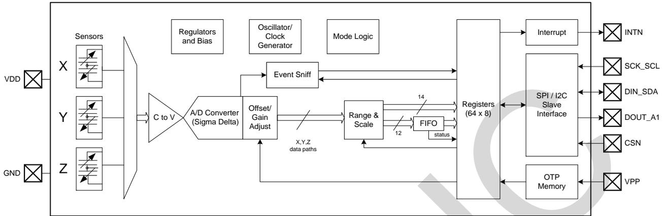
Figure 1. Block Diagram
