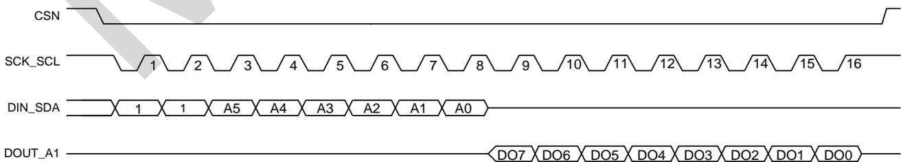
Figure 19. SPI Register Read Cycle - Single
