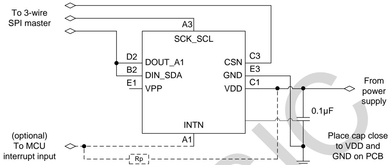
NOTE Rp: Attach typical 4.7kΩ pullup resistor if INTN is defined as open-drain.
