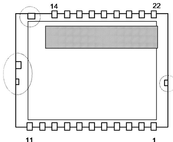
1. Pad layout and size can modify by customers material, equipment, and method. Please adjust pad layout according to your conditions.
