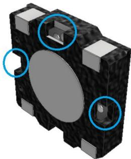
For best frequency response results, fill in these vent holes after reflow or hand soldering to prevent potential cancelation.
