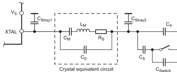
Using  $C_4 = 9.2\text{pF} \pm 2\%$ ,  $C_5 = 6.8\text{pF} \pm 5\%$ , a switch port with  $C_{Switch} = 3\text{pF} \pm 10\%$ , stray capacitances on each side of the crystal of  $C_{Stray1} = C_{Stray2} = 1\text{pF} \pm 10\%$ , a parallel capacitance of the crystal of  $C_0 = 3.2\text{pF} \pm 10\%$  and a crystal with  $C_M = 13\text{fF} \pm 10\%$ , an FSK deviation of  $\pm 21\text{kHz}$  typical with worst case tolerances of  $\pm 16.3\text{kHz}$  to  $\pm 28.8\text{kHz}$  results.
