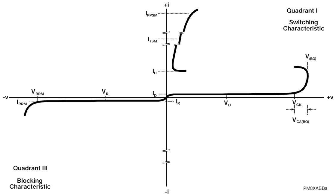
Figure 2. TISP8201HDM AK Terminal Characteristic
