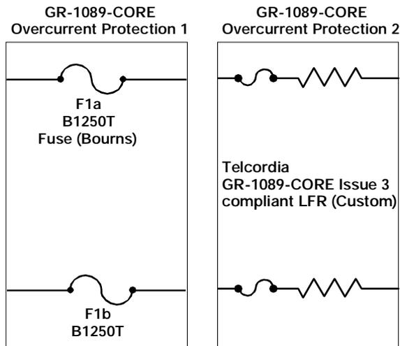
Figure 4. Typical Overcurrent Protection
