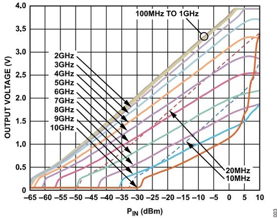
Figure 3. Typical  $V_{RMS}$  vs. Input Power (dBm) vs. Frequency (10 MHz to 10 GHz) at  $25^\circ$ C
