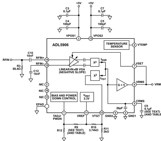
Figure 51. Basic Connections for Operation in Measurement Mode
