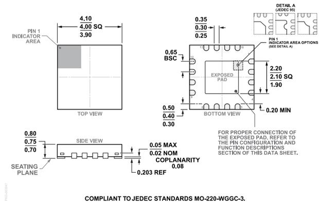
Figure 66. 16-Lead Lead Frame Chip Scale Package [LFCSP\_WQ]
