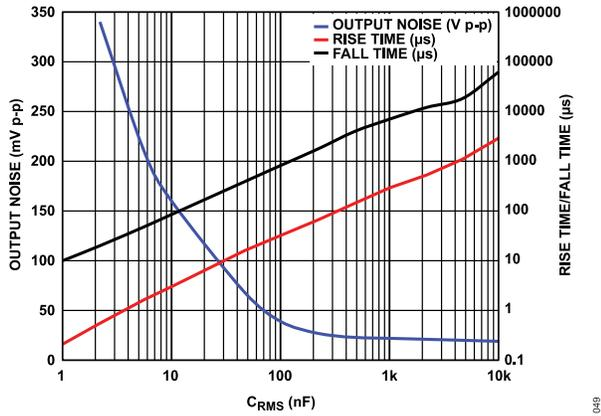
Figure 50 also shows how the response time is affected by the value of  $C_{RMS}$ . To measure this, an RF burst at 2.14 GHz at 0 dBm was applied to the ADL5906. The 10% to 90% rise time and 90% to 10% fall time were then measured.
