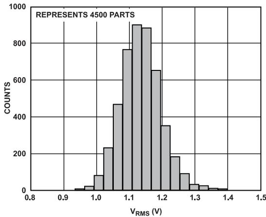
Figure 28. Distribution of  $V_{RMS}$ ,  $P_{IN} = -45$  dBm, 900 MHz
