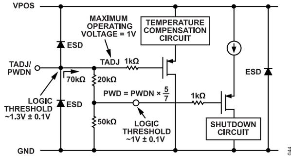
Figure 46. TADJ/PWDN Interface Simplified Schematic
