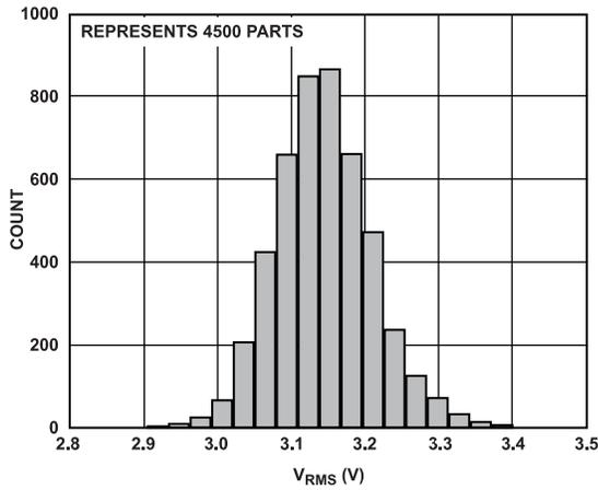
Figure 27. Distribution of  $V_{RMS}$ ,  $P_{IN} = -10$  dBm, 900 MHz
