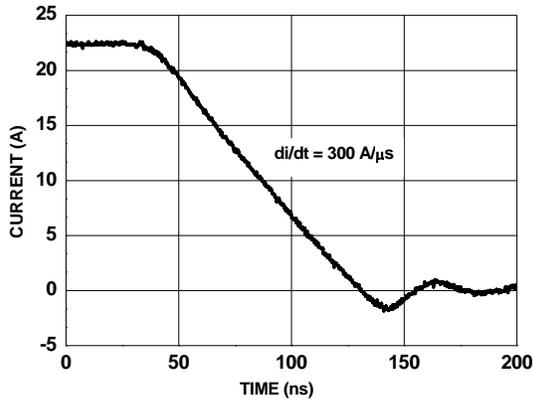
Figure 13. FDMC2514SDC SyncFET body diode reverse recovery characteristic
