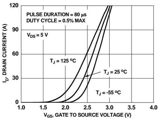
**Figure 5. Transfer Characteristics**
