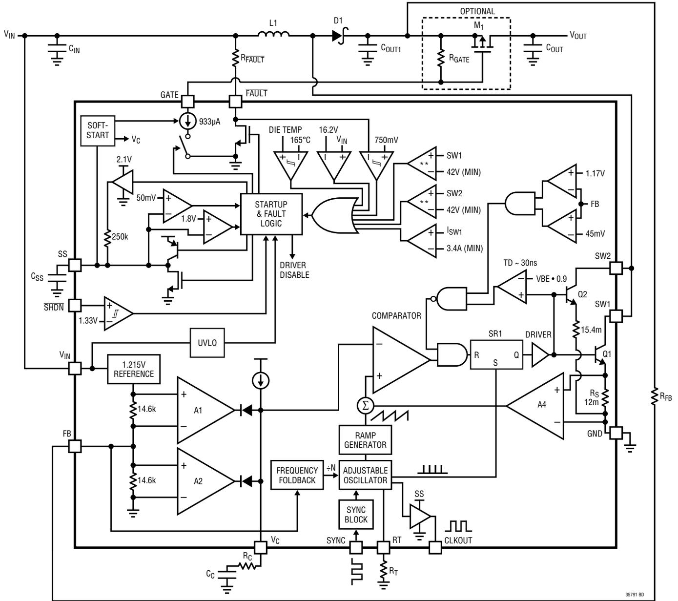
\*\* SW OVERVOLTAGE PROTECTION IS NOT GUARANTEED TO PROTECT THE LT3579/LT3579-1 DURING SW OVERVOLTAGE EVENTS.
