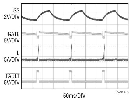
Figure 5. Continuous Output Short Showing  $\overline{\text{FAULT}}$  Timeout Cycle
