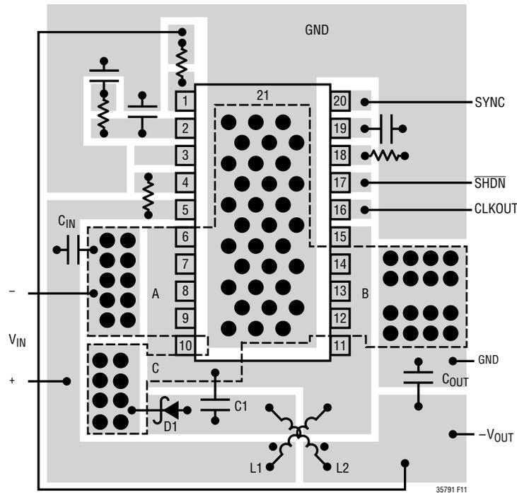
A- RETURN  $C_{IN}$  GROUND DIRECTLY TO LT3579 EXPOSED PAD PIN 21. IT IS ADVISED TO NOT COMBINE  $C_{IN}$  GROUND WITH GND EXCEPT AT THE EXPOSED PAD.
