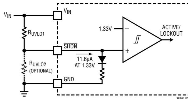
Figure 3. Configurable UVLO
