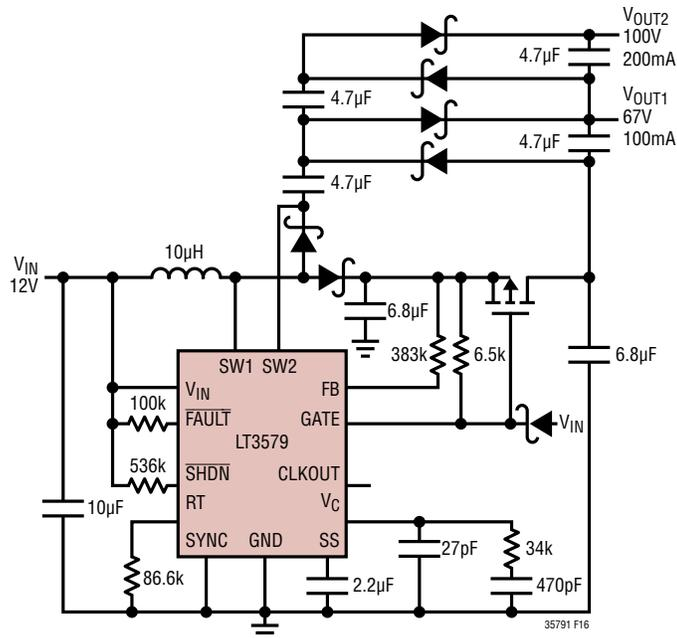
Figure 16. High  $V_{OUT}$  Charge Pump Topology
