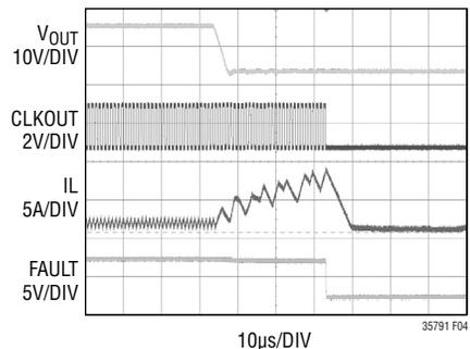
Figure 4. Output Short Circuit Protection of the LT3579
