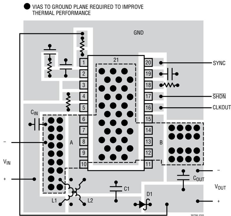
A- RETURN  $C_{IN}$  AND L2 GROUND DIRECTLY TO LT3579 EXPOSED PAD PIN 21. IT IS ADVISED TO NOT COMBINE  $C_{IN}$  AND L2 GROUND WITH GND EXCEPT AT THE EXPOSED PAD.
