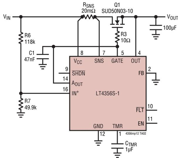
24V Overvoltage Regulator Withstands 150V at VIN
