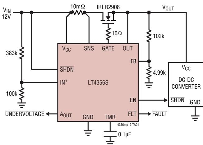
Overvoltage Protector Regulates Output at 27V During Transient
