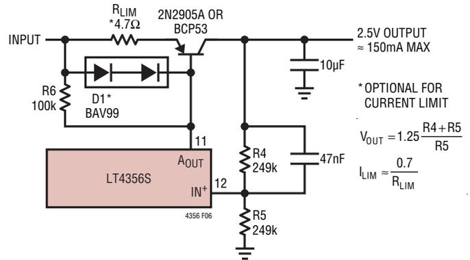
Figure 6. Auxiliary LDO Output with Optional Current Limit
