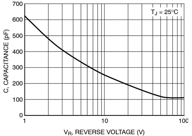
Figure 4. Typical Capacitance
