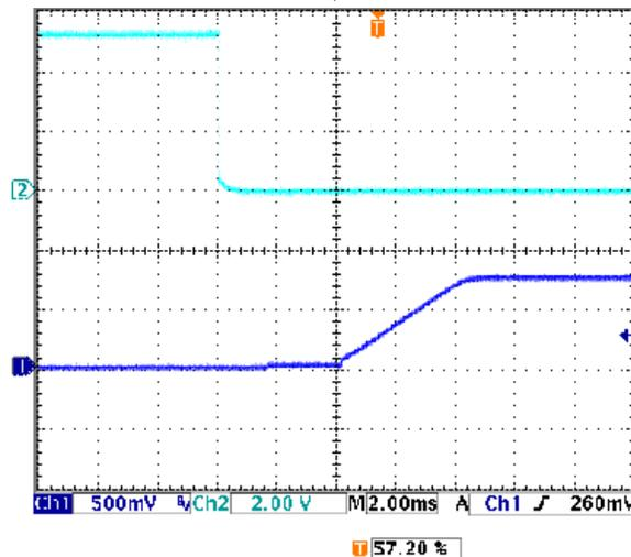
Step Load Transient Response (Vin=5V, Vout=0.75V, Cload=0, Iout=8A to 16A)
