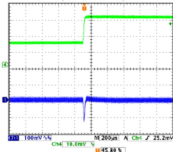
Step Load Transient Response (Vin=5V, Vout=0.75V, Cload=0, Iout=16A to 8A)
