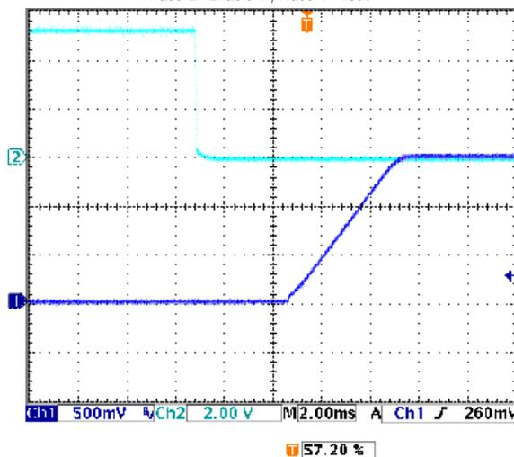
Step Load Transient Response (V<sub>in</sub>=5V, V<sub>out</sub>=1.5V, Cload=0, I<sub>out</sub>=8A to 16A)
