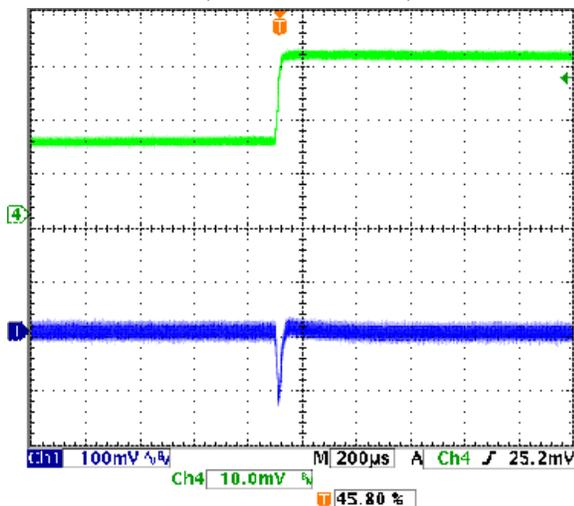
Step Load Transient Response (Vin=5V, Vout=3.3V, Cload=0, Iout=16A to 8A)
