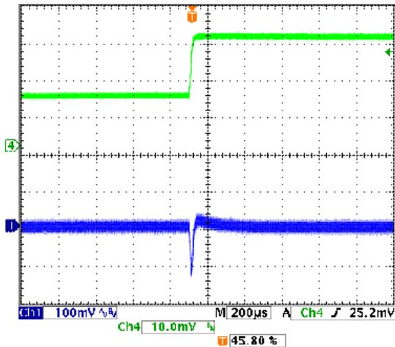
Step Load Transient Response ( $V_{in}=5V, V_{out}=2.5V, \text{Load}=0, I_{out}=16A \text{ to } 8A$ )
