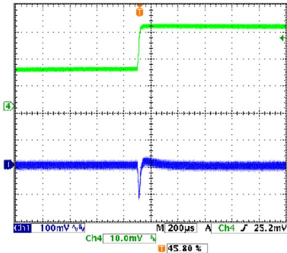
Step Load Transient Response (V<sub>in</sub>=5V, V<sub>out</sub>=1.8V, C<sub>load</sub>=0, I<sub>out</sub>=16A to 8A)
