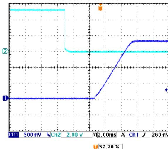
Step Load Transient Response (V<sub>in</sub>=5V, V<sub>out</sub>=1.8V, C<sub>load</sub>=0, I<sub>out</sub>=8A to 16A)
