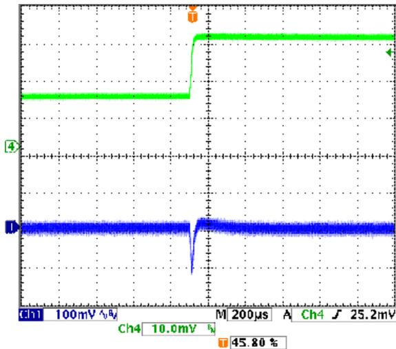
Step Load Transient Response (V<sub>in</sub>=5V, V<sub>out</sub>=1.5V, Cload=0, I<sub>out</sub>=16A to 8A)
