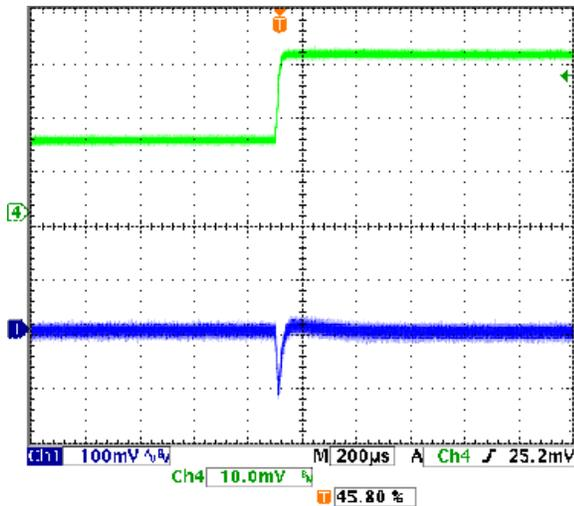
Step Load Transient Response ( $V_{in}=5V, V_{out}=1.2V, C_{load}=0, I_{out}=16A$  to  $8A$ )
