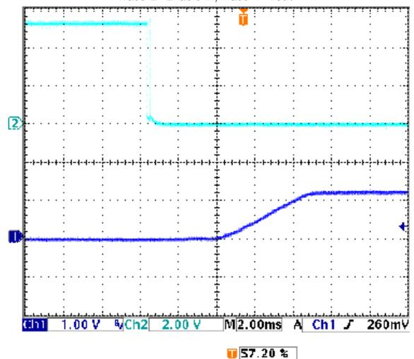
Step Load Transient Response ( $V_{in}=5V, V_{out}=1.2V, C_{load}=0, I_{out}=8A$  to  $16A$ )
