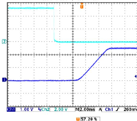
Step Load Transient Response ( $V_{in}=5V, V_{out}=2.5V, \text{Load}=0, I_{out}=8A \text{ to } 16A$ )
