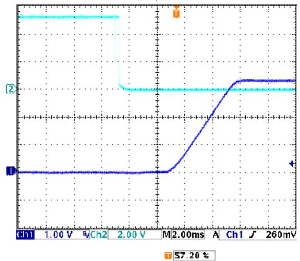
Step Load Transient Response (Vin=5V, Vout=3.3V, Cload=0, Iout=8A to 16A)
