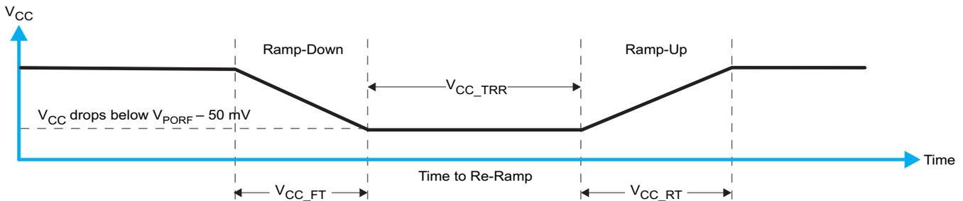
Figure 19. V<sub>CC</sub> is Lowered Below the POR Threshold, Then Ramped Back Up to V<sub>CC</sub>
