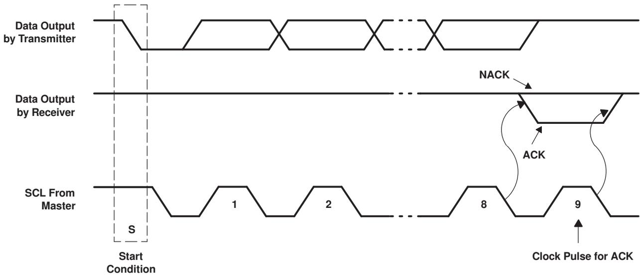
Figure 10. Acknowledgment on the I<sup>2</sup>C Bus
