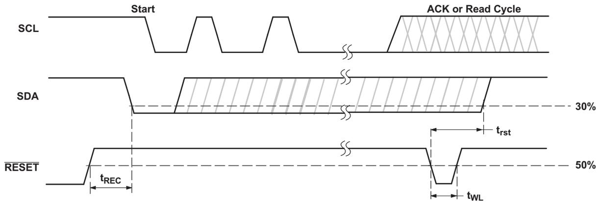
**Figure 6. Reset Timing**
