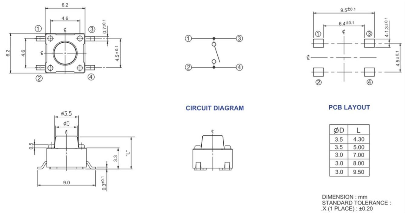
Figure 2 – Through-Hole, 222AD, Vertical Actuation
