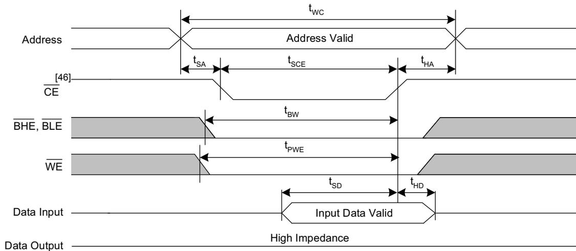
Figure 16. SRAM Write Cycle 3:  $\overline{BHE}$ ,  $\overline{BLE}$  Controlled<sup>[42, 43, 44, 45, 47]</sup>
