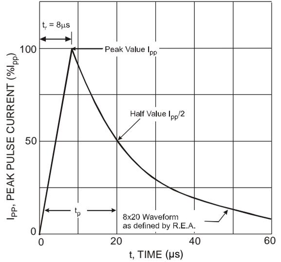
Figure 2 Typical 8 x 20µs Pulse Waveform
