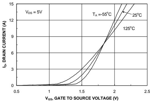
Figure 5. Transfer Characteristics.
