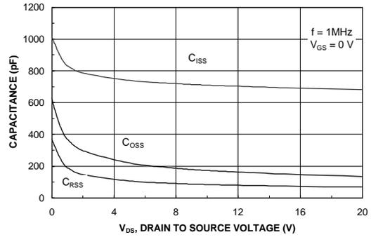
Figure 8. Capacitance Characteristics.
