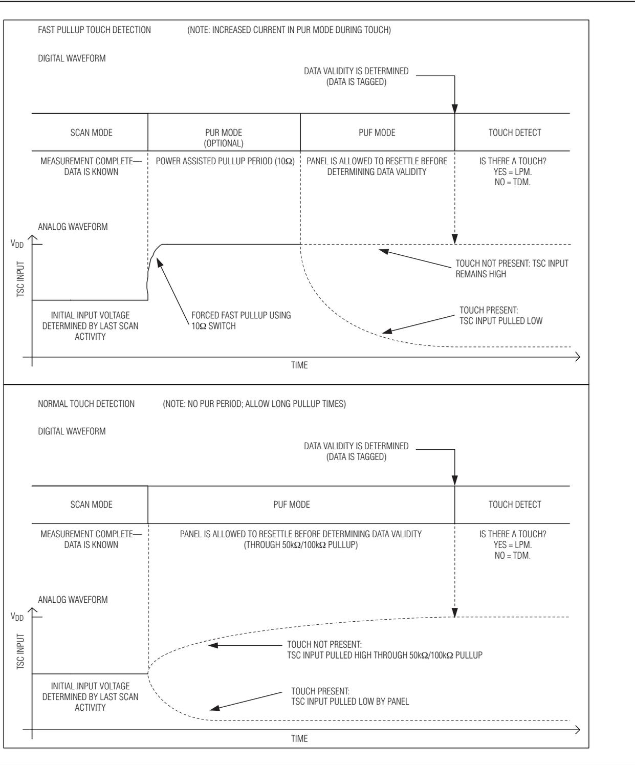
Figure 7. Touch-Detection Operations
