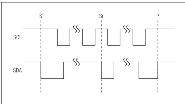
Figure 23. START, STOP, and Repeated START Conditions
