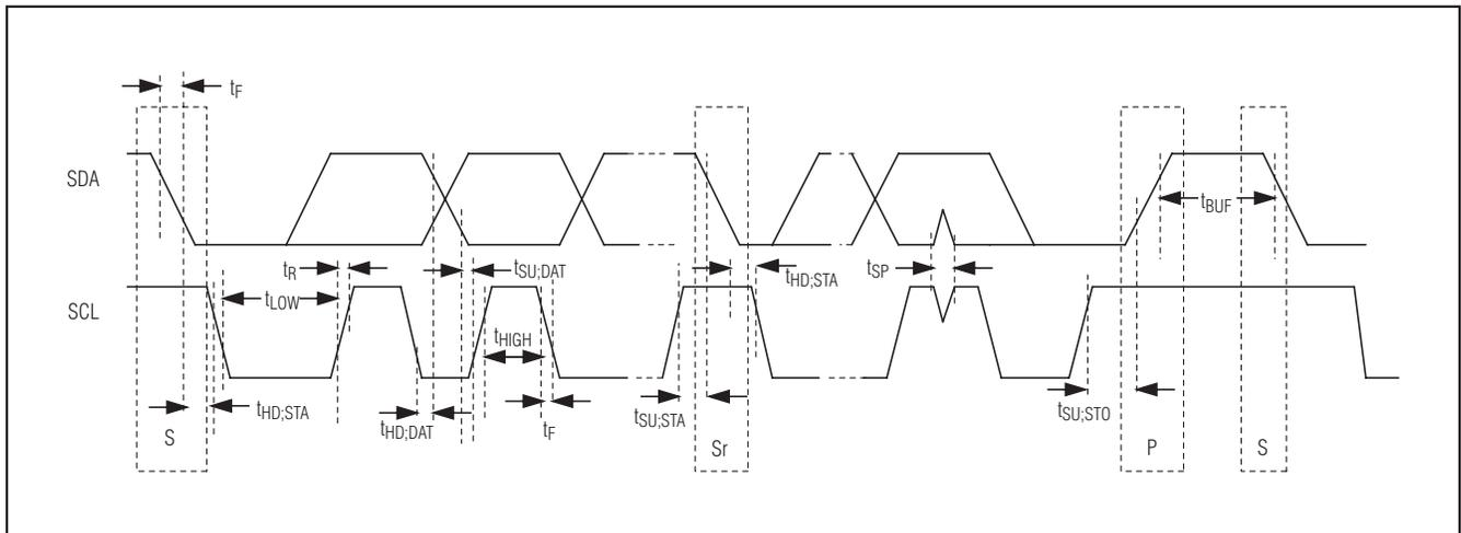
Figure 1. I<sup>2</sup>C Timing Diagram
