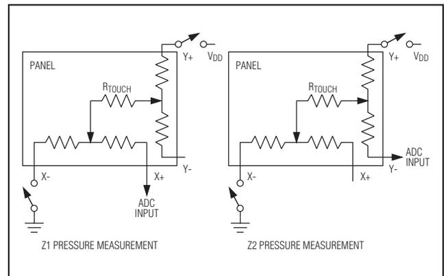
Figure 5. Pressure Measurements
