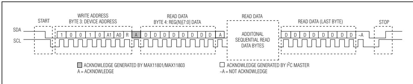
Figure 29. I<sup>2</sup>C Streamlined Read Sequence
