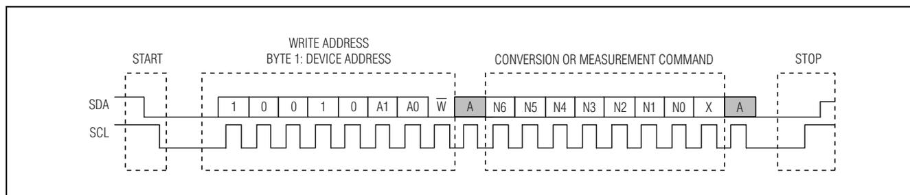
Figure 30. I<sup>2</sup>C Conversion and Measurement Commands
