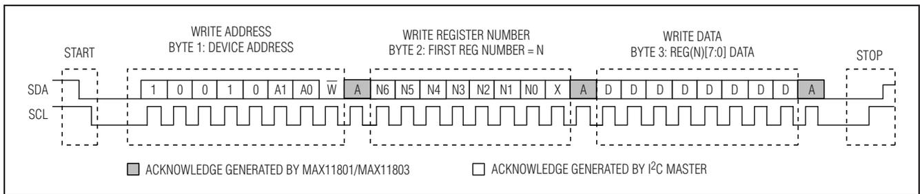
Figure 25. I<sup>2</sup>C Single Write Sequence
