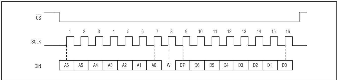
Figure 17. SPI Single Configuration Register Write Sequence—MAX11800/MAX11802
