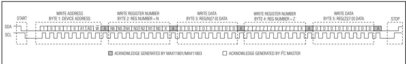
Figure 26. I<sup>2</sup>C Multiple Write Sequence
