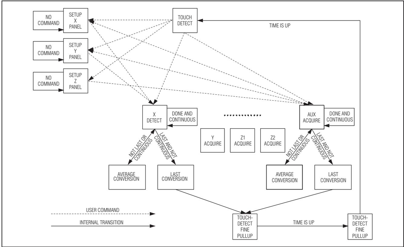
Figure 8. State Machine Transitions (Direct Conversion Mode)—MAX11800–MAX11803
