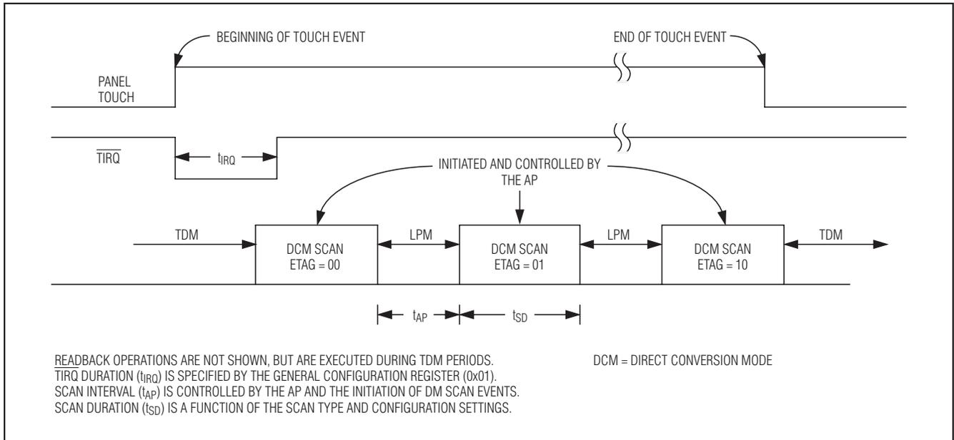
Figure 10. Edge Interrupt Mode (Direct Conversion Mode)—MAX11800–MAX11803
