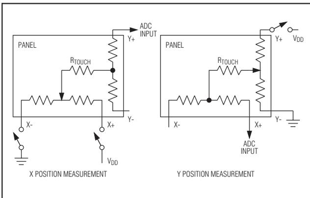
Figure 4. Position Measurements
