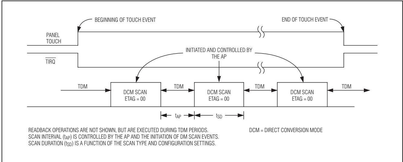
Figure 9. Continuous Interrupt Mode (Direct Conversion Mode)
