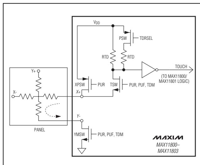
Figure 6. Touch-Detection Circuitry
