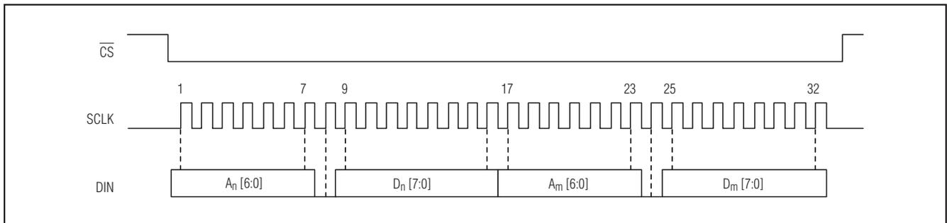
Figure 18. SPI Multiple Configuration Register Write Sequence—MAX11800/MAX11802
