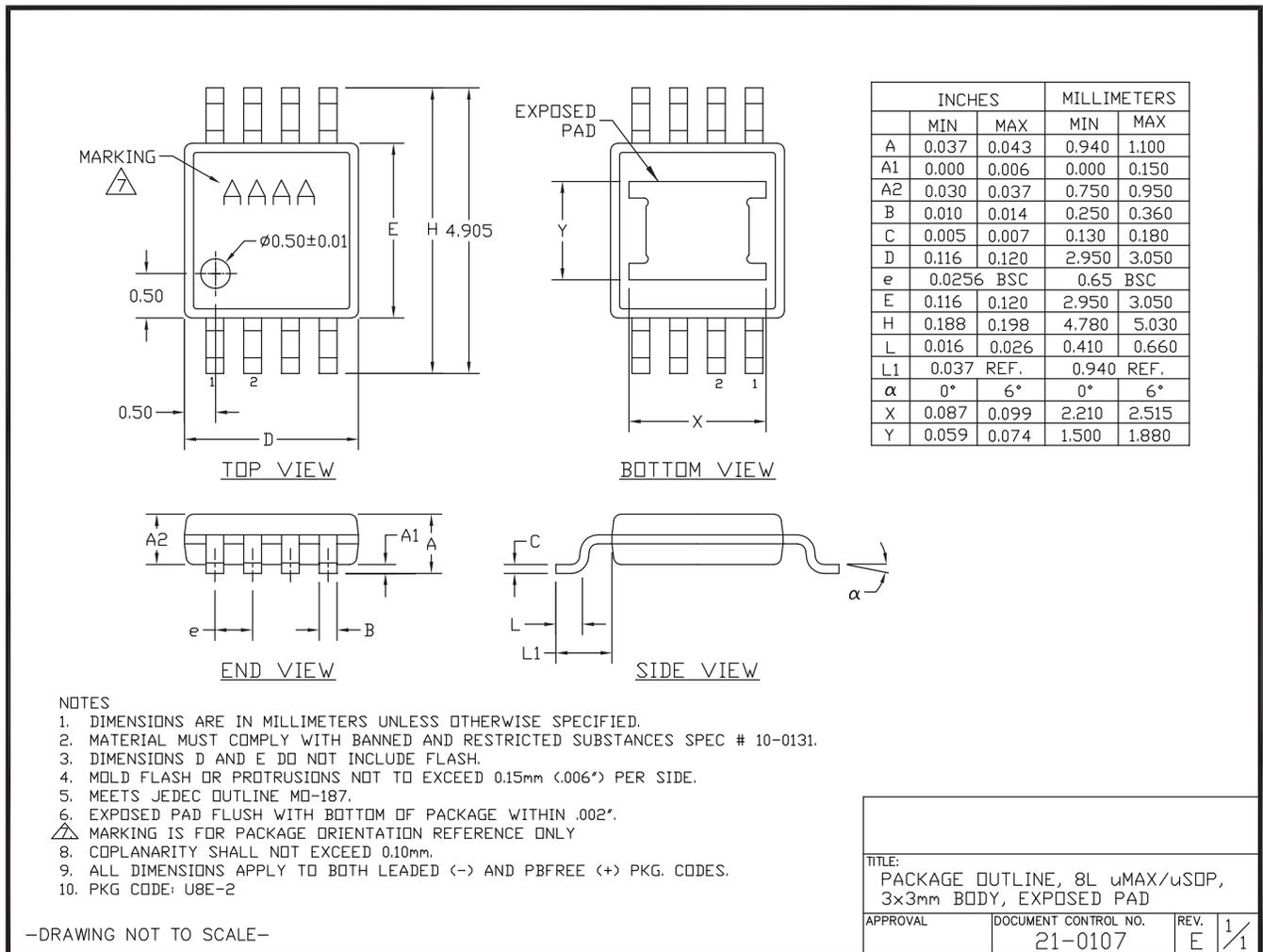
**Note:** The MAX1806 has an exposed thermal pad on the bottom side of the package.
