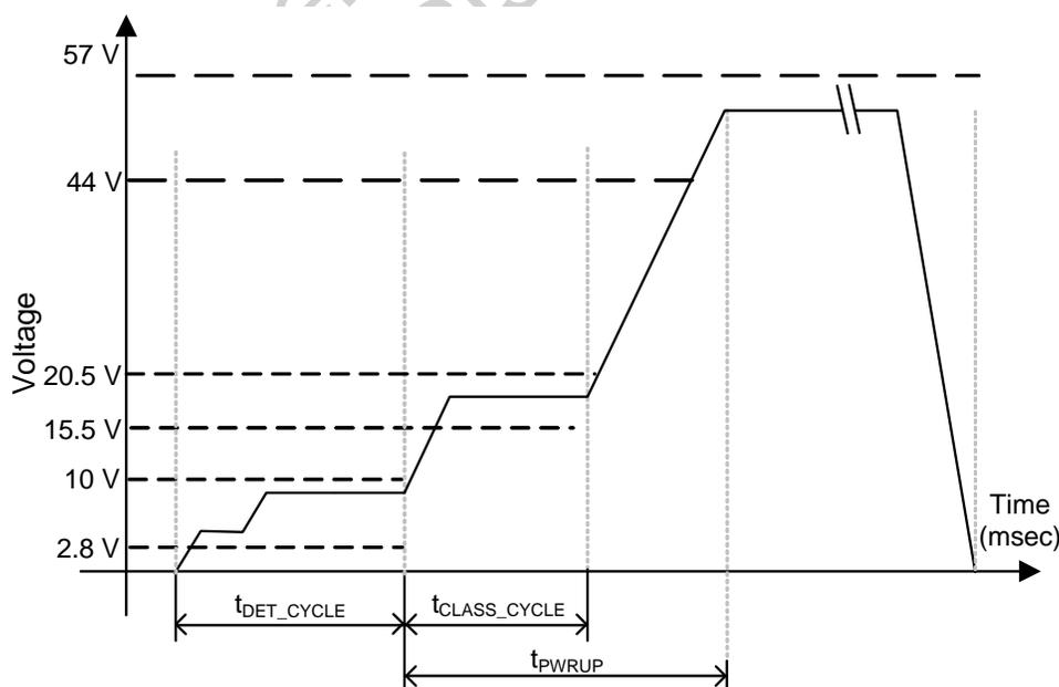
**Figure 2. Detection, Classification, Powerup, and Disconnect Sequence**
