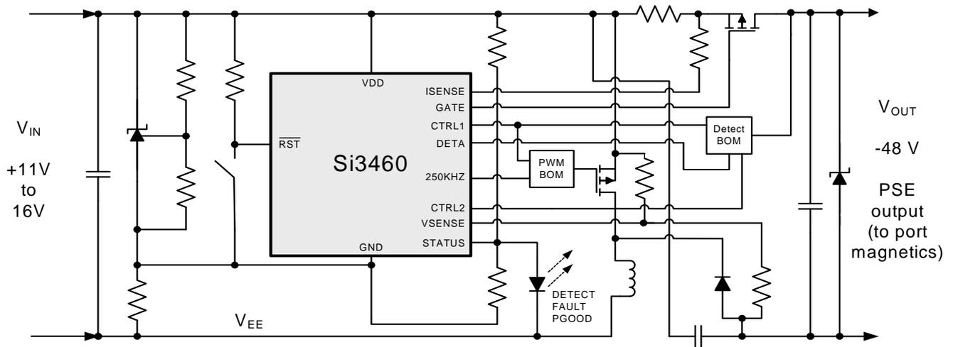
Note: Refer to the Si3460-EVB User Guide for complete schematic details
