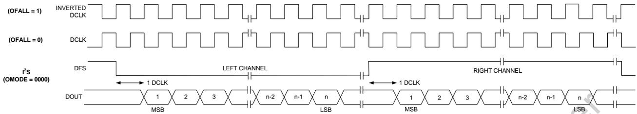
**Figure 8. I<sup>2</sup>S Digital Audio Format**
