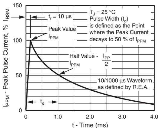
Fig. 3 - Pulse Waveform
