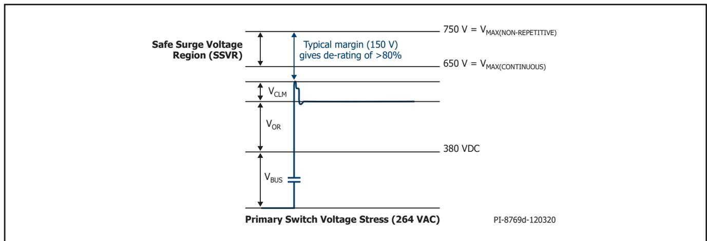
Figure 20. Peak Drain Voltage for 264 VAC Input Voltage.
