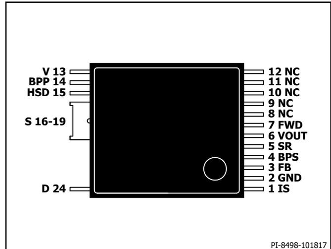
Figure 5. Pin Configuration.
