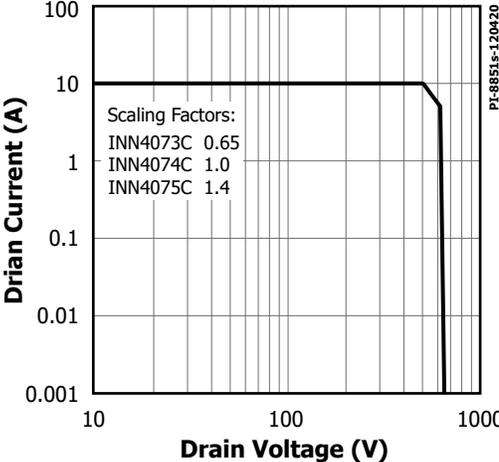
Figure 24. Maximum Allowable Drain Current vs. Drain Voltage.
