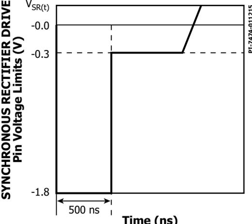
Figure 25. SYNCHRONOUS RECTIFIER DRIVE Pin Negative Voltage.
