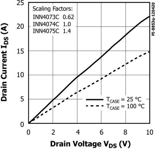
Figure 21. Output Characteristics.
