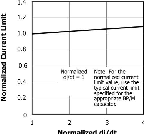
Figure 26. Standard Current Limit vs.  $di/dt$ .
