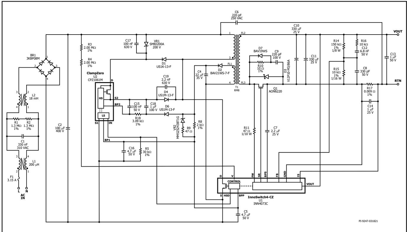
Figure 8. Schematic 20 V / 3.25 A Notebook Adapter Power Supply.
