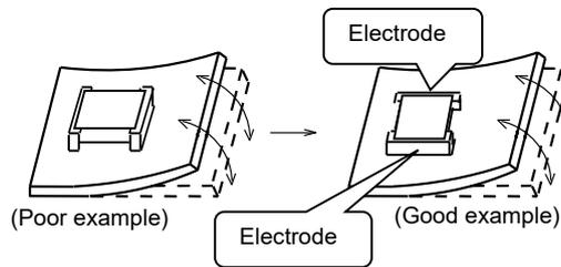
(2) Components location on PCB separation
