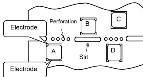
(3) Mounting components near screw holes
