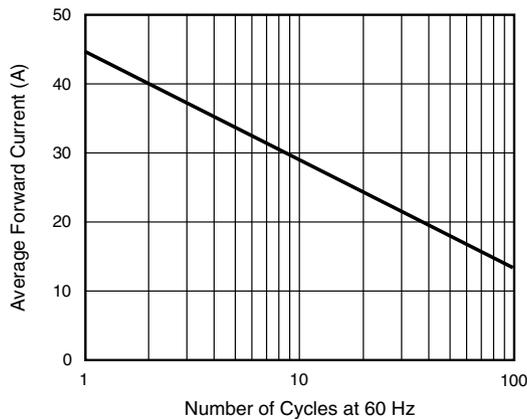
Fig. 3 - Maximum Non-Repetitive Peak Forward Surge Current
