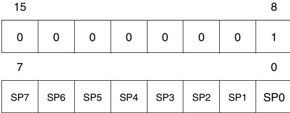
The Stack Pointer is a 16-bit register which is always pointing to the next free location in the stack. It is then decremented after data has been pushed onto the stack and incremented before data is popped from the stack (see Figure 8).
