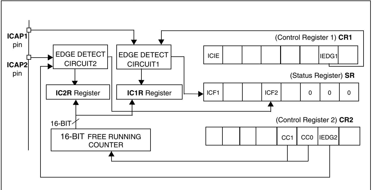
Figure 40. Input Capture Timing Diagram
