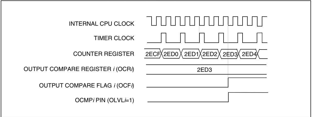
Figure 43. Output Compare Timing Diagram,  $f_{\text{TIMER}} = f_{\text{CPU}}/4$
