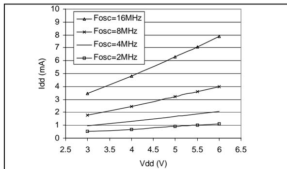
Figure 68. Typical  $I_{DD}$  in WAIT at  $T_A=25^\circ\text{C}$
