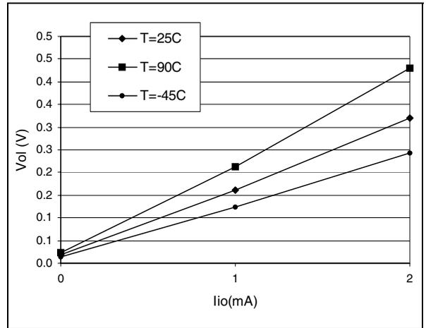
Figure 81. Typ.  $V_{OL}$  at  $V_{DD}=3V$  (high-sink)
