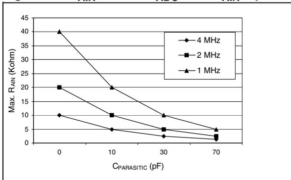
Figure 98. Recommended C<sub>AIN</sub>/R<sub>AIN</sub> values<sup>3)</sup>
