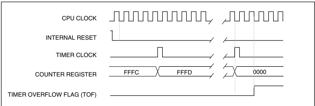
**Note:** The Device is in reset state when the internal reset signal is high, when it is low the Device is running.
