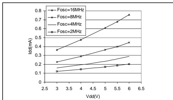
Figure 69. Typ.  $I_{DD}$  in SLOW-WAIT at  $T_A=25^\circ\text{C}$
