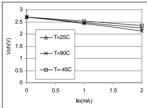
Figure 86. Typ.  $V_{OH}$  at  $V_{DD}=3V$
