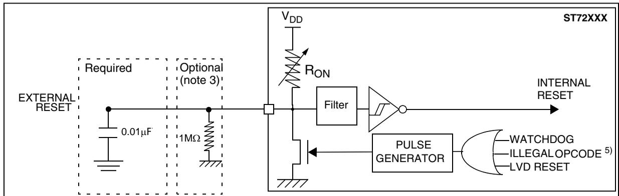
Figure 92.  $\overline{\text{RESET}}$  pin protection when LVD is disabled.<sup>1)</sup>
