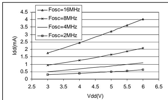
Figure 67. Typical  $I_{DD}$  in SLOW at  $T_A=25^\circ\text{C}$
