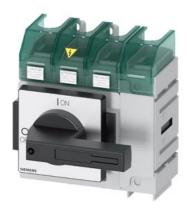
SENTRON, Molded case switch 3LD5 UL, Main switch, 4-pole, certified according to UL489 UL60947-4-1 and IEC60947-3, UL: 125A, SCCR 65kA at 480VAC, Operating power at 480VAC 3-phase: 75hp, IEC: 125A, Operating power at AC-23A at 400V: 55kW, floor mounting with direct handle, black, incl. terminal covers for the infeed side
