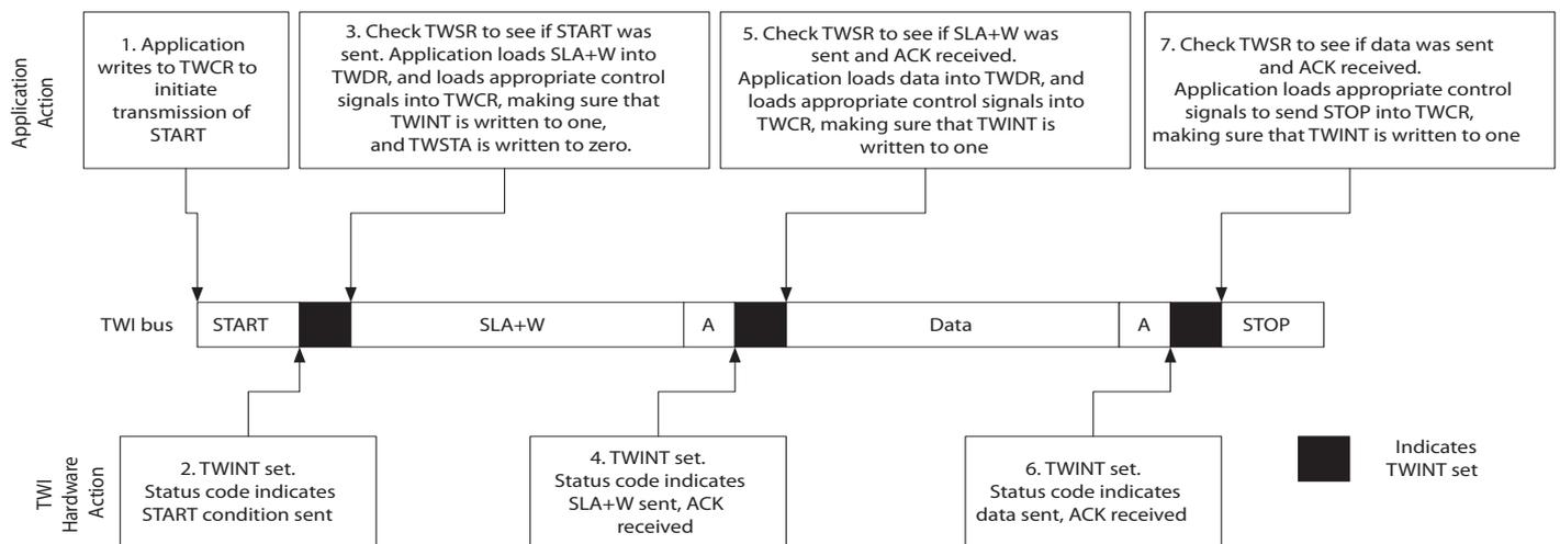
1. The first step in a TWI transmission is to transmit a START condition. This is done by writing a specific value into TWCR, instructing the TWI hardware to transmit a START condition. The value to write is described later on. However, it is important that the TWINT bit is set in the value written. Writing a one to TWINT clears the flag. The TWI will not start any operation as long as the TWINT bit in TWCR is set. Immediately after
