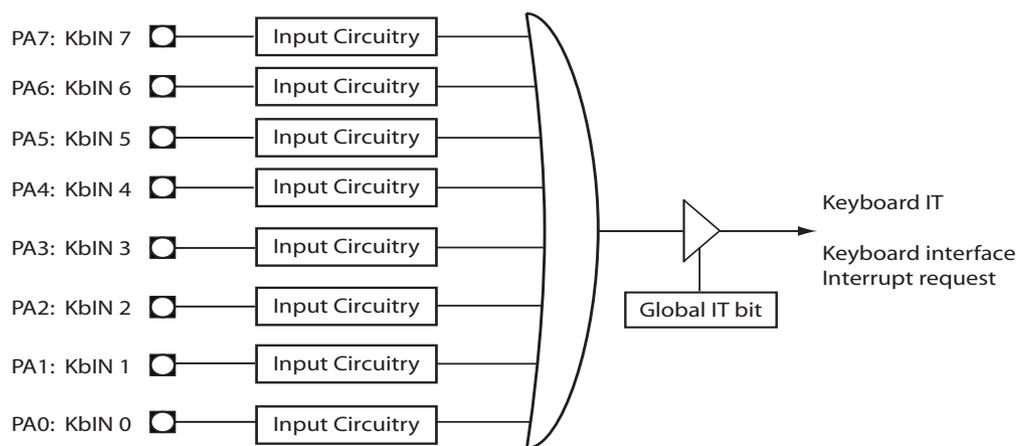
**Figure 23-2. Keyboard Input Circuitry**
