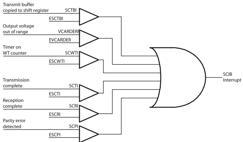
This signal is high level active. Each of the sources is able to activate the SCIB interruption which is cleared by software by clearing the corresponding bits in the Smart Card Interrupt register.
