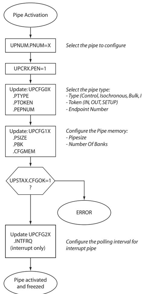
Once the Pipe is activated (UPCRX.PEN set), the hardware is ready to send requests to the Device.
