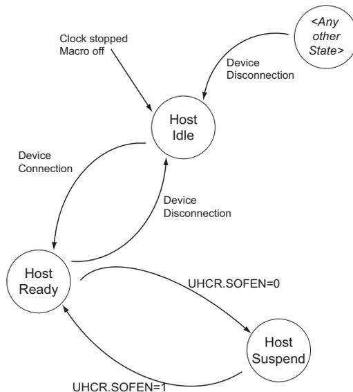
USB Host controller state after an hardware reset is 'Reset'. When the USB Host controller is enabled, the USB controller is in 'Idle' state. In this state, the USB Host controller waits for the Device connection, **with a minimum power consumption**. The USB Pad should be in Idle mode. The macro does not need to have the PLL activated to enter in 'Host Ready' state.
