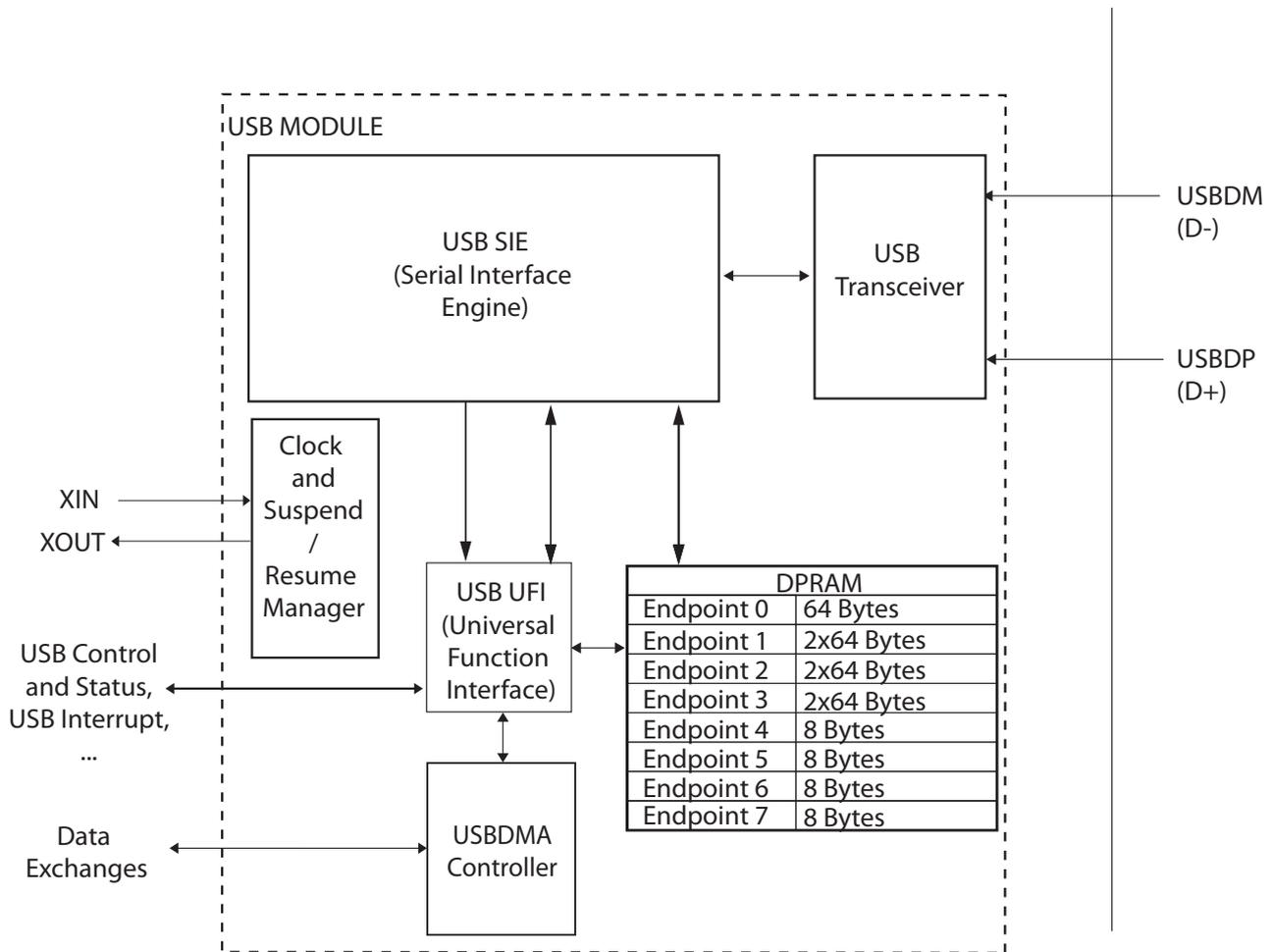
The USB module of the AT90SCR100 is made up of the following elements:
