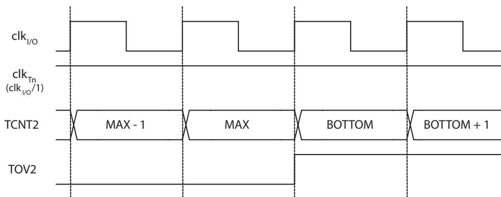
Figure 13-33 shows the same timing data, but with the prescaler enabled.
