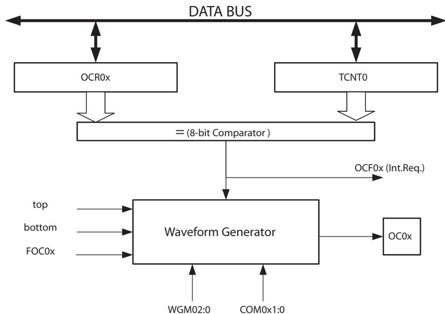
The OCR0x Registers are double buffered when using any of the Pulse Width Modulation (PWM) modes. For the normal and Clear Timer on Compare (CTC) modes of operation, the dou-
