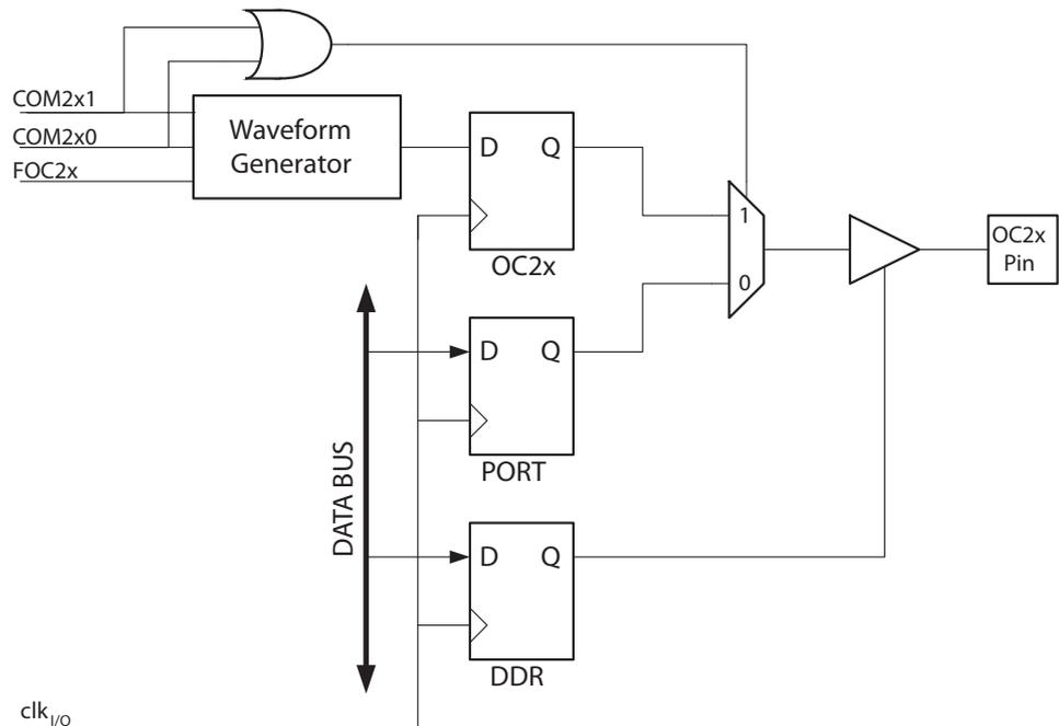
The general I/O port function is overridden by the Output Compare (OC2x) from the Waveform Generator if either of the COM2x1:0 bits are set. However, the OC2x pin direction (input or output) is still controlled by the Data Direction Register (DDR) for the port pin. The Data Direction Register bit for the OC2x pin must be set as output before the OC2x value is visible on the pin. The port override function is independent of the Waveform Generation mode.
