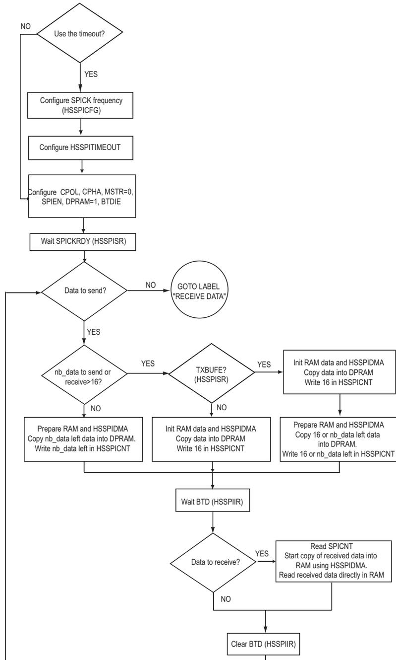
**Figure 21-7. SPI - Slave with DPRAM operation - Second part**
