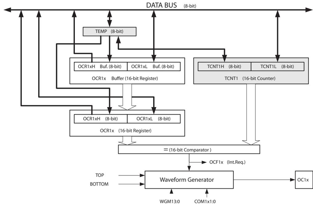
The OCR1x Register is double buffered when using any of the twelve *Pulse Width Modulation* (PWM) modes. For the Normal and *Clear Timer on Compare* (CTC) modes of operation, the double buffering is disabled. The double buffering synchronizes the update of the OCR1x Compare Register to either TOP or BOTTOM of the counting sequence. The synchronization prevents the occurrence of odd-length, non-symmetrical PWM pulses, thereby making the output glitch-free.
