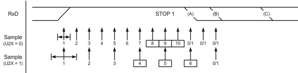
The same majority voting is done to the stop bit as done for the other bits in the frame. If the stop bit is registered to have a logic 0 value, the Frame Error (FE0) Flag will be set.
