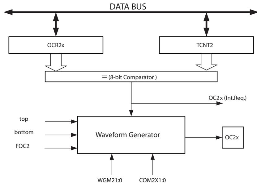
The OCR2x Register is double buffered when using any of the Pulse Width Modulation (PWM) modes. For the Normal and Clear Timer on Compare (CTC) modes of operation, the double buffering is disabled. The double buffering synchronizes the update of the OCR2x Compare Register to either top or bottom of the counting sequence. The synchronization prevents the occurrence of odd-length, non-symmetrical PWM pulses, thereby making the output glitch-free.
