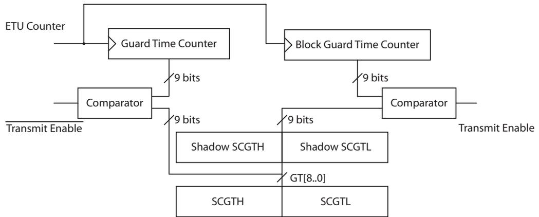
To illustrate the use of Guard Time and Block Guard Time, consider the ISO/IEC7816-3 recommendation : Guard Time = 2 (minimum delay between 2 consecutive characters sent by the Terminal = 12 ETUs), and Block Guard Time = 22 ETUs.
