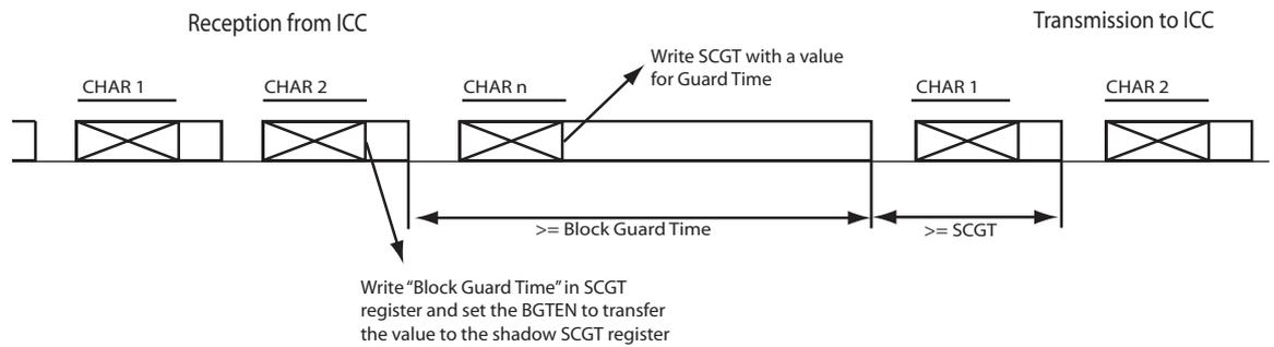
**Figure 15-4.** Guard Time and Block Guard Time counters
