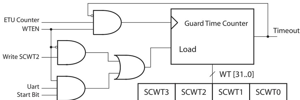
In the so called manual mode, the counter is loaded, if WTEN = 0, during the write of SCWT2 register. The counter is loaded with a 32 bit word built with SCWT3 SCWT2 SCWT1 SCWT0 registers (SCWT0 contains WT[7-0] bytes. WTEN is located in the SCICR register.
