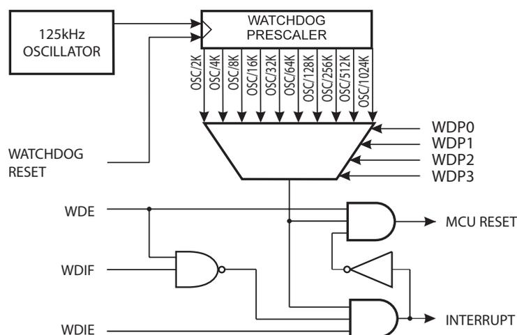
The Watchdog Timer (WDT) is a timer counting cycles of a separate on-chip 125 kHz oscillator. The WDT gives an interrupt or a system reset when the counter reaches a given time-out value. In normal operation mode, it is required that the system uses the WDR - Watchdog Timer Reset - instruction to restart the counter before the time-out value is reached. If the system doesn't restart the counter, an interrupt or system reset will be issued.
