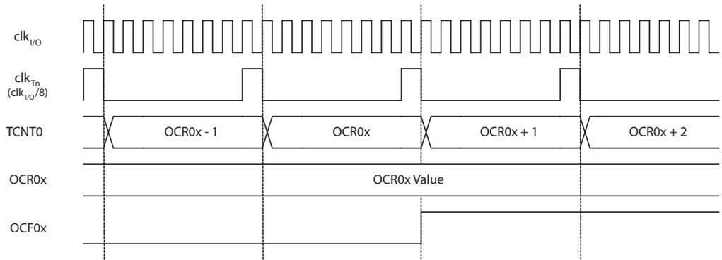
Figure 13-11 shows the setting of OCF0A and the clearing of TCNT0 in CTC mode and fast PWM mode where OCR0A is TOP.
