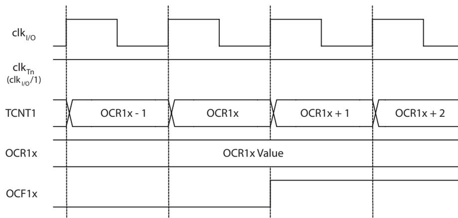
[Figure 13-22](#) shows the same timing data, but with the prescaler enabled.
