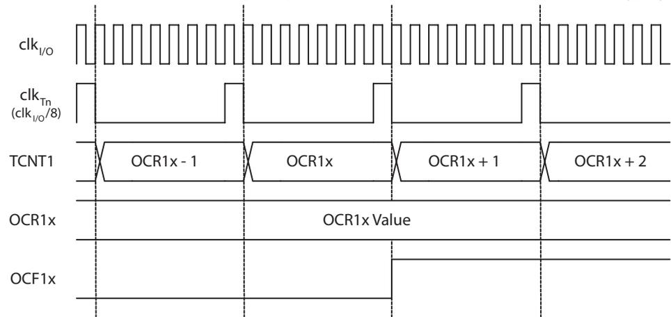
Figure 13-23 shows the count sequence close to TOP in various modes. When using phase and frequency correct PWM mode the  $OCR1x$  Register is updated at BOTTOM. The timing diagrams will be the same, but TOP should be replaced by BOTTOM, TOP-1 by BOTTOM+1 and so on. The same renaming applies for modes that set the TOV1 Flag at BOTTOM.
