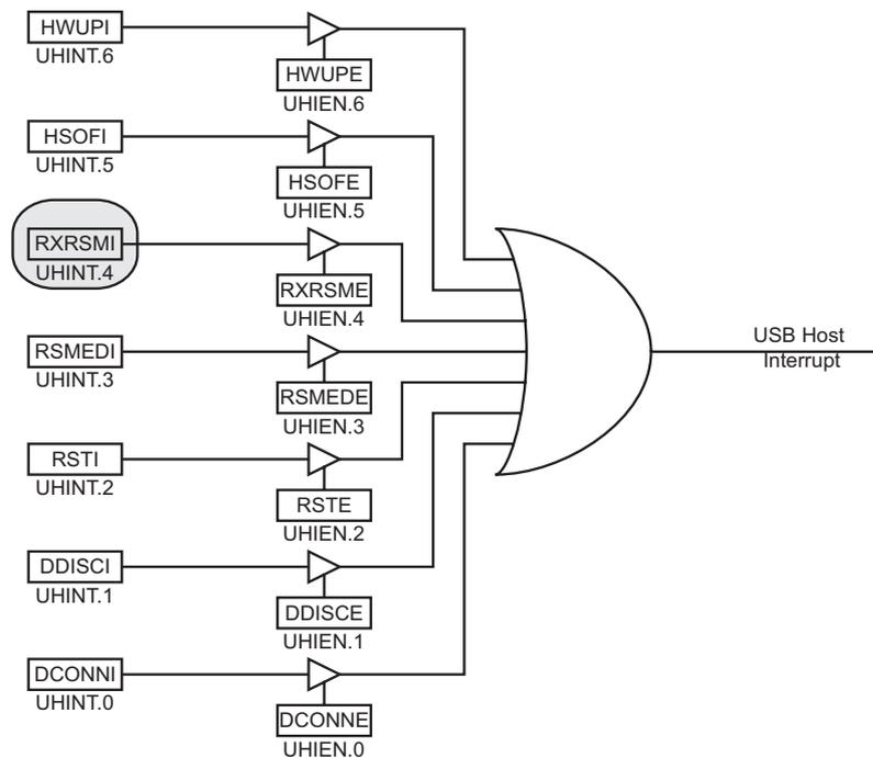
Figure 17-10. USB Host Controller Pipe Interrupt System
