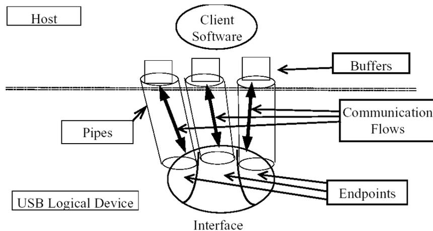
In the USB Host controller, a Pipe will be associated to a Device Endpoint, considering the Device Configuration Descriptors.
