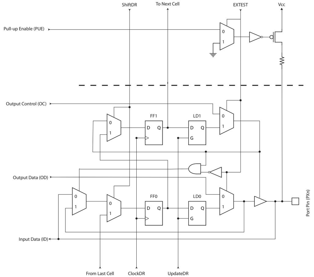
Figure 27-4. General Port Pin Schematic Diagram
