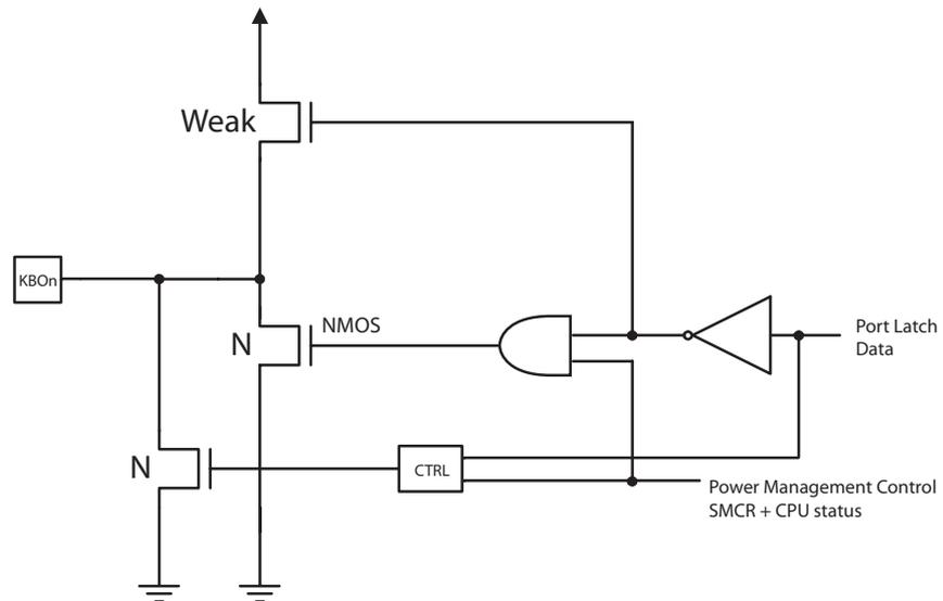
The current limitation of the CTRL block requires a polarisation current of about 250µA. This block is automatically disabled in power-down, power-save, standby and extended standby modes.
