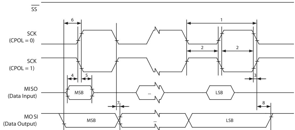
**Figure 31-3. SPI Interface Timing Requirements (Slave Mode)**
