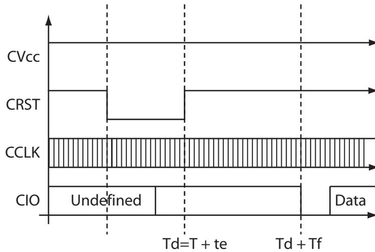
The removal of the smart card will automatically start the power off sequence as described in [Figure 15-10](#).
