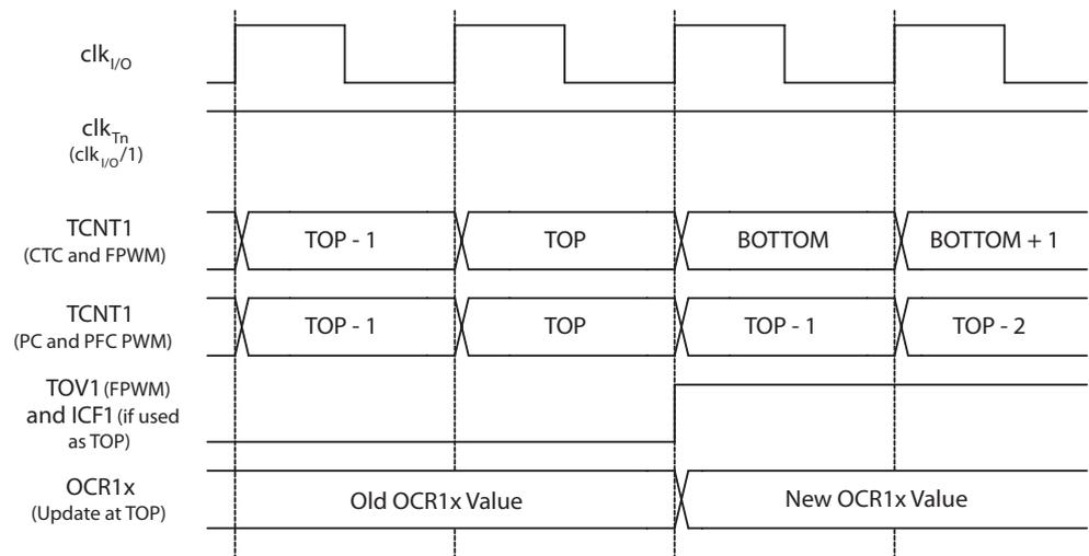
Figure 13-24 shows the same timing data, but with the prescaler enabled.
