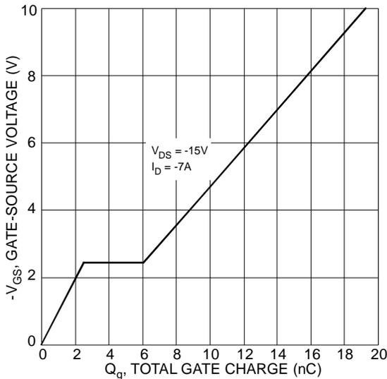
Figure 11 Gate-Charge Characteristics
