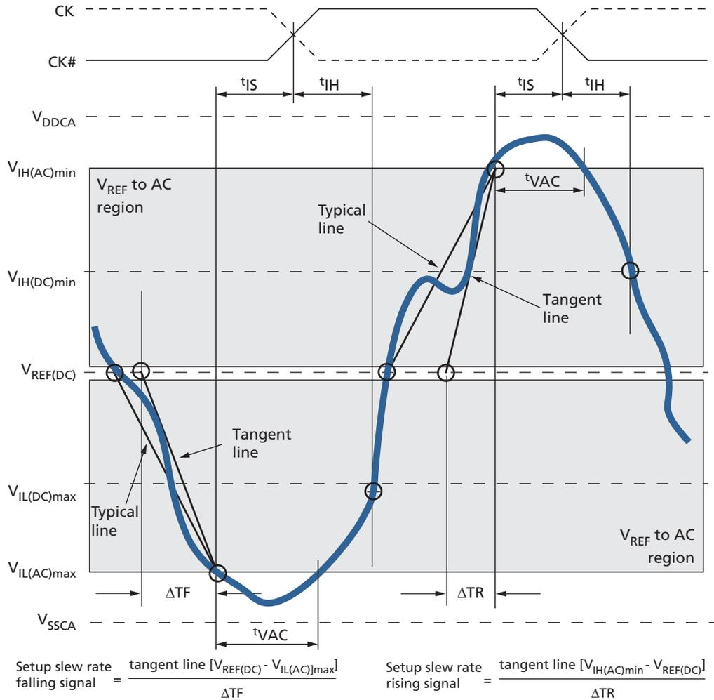
**Figure 82: Tangent Line – t<sub>IH</sub> for CA and CS# Relative to Clock**
