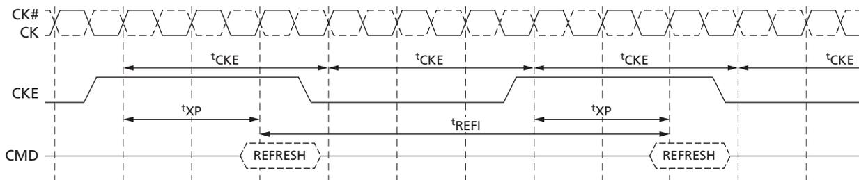
Note: 1. The pattern shown can repeat over an extended period of time. With this pattern, all AC and DC timing and voltage specifications with temperature and voltage drift are ensured.
