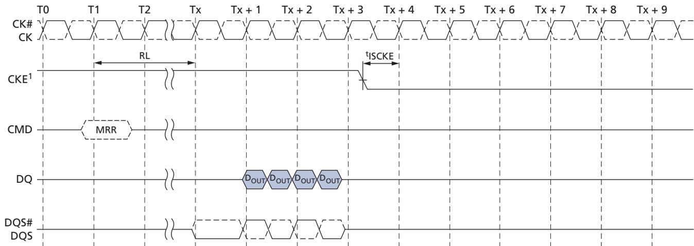
Note: 1. CKE can be registered LOW at  $(RL + RU(t_{DQ\text{SCK}}/t_{\text{CK}}) + BL/2 + 1)$  clock cycles after the clock on which the MRR command is registered.
