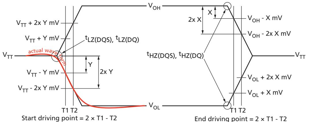
7. Measured from the point when DQS/DQS# begins driving the signal, to the point when DQS/DQS# begins driving the first rising strobe edge.
