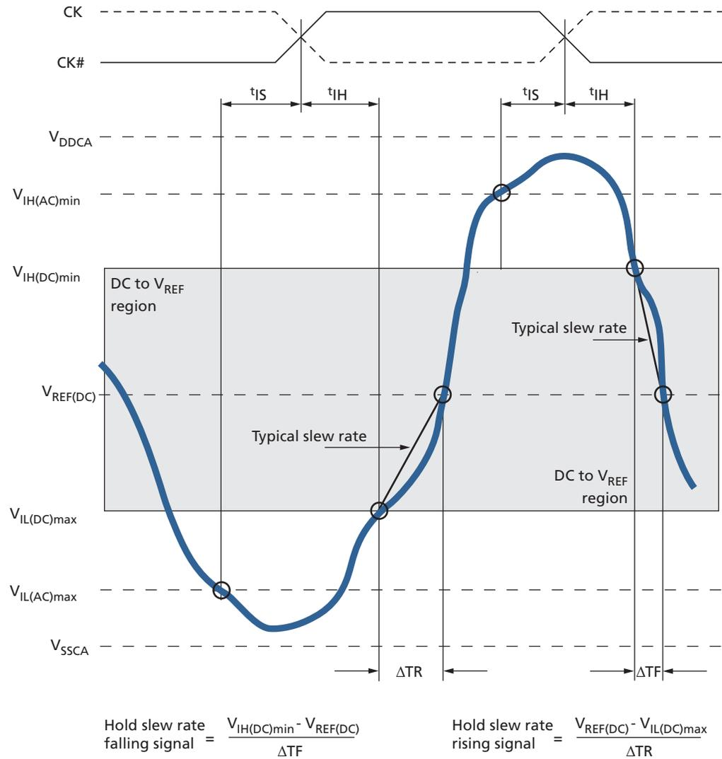
**Figure 81: Tangent Line – t<sub>IS</sub> for CA and CS# Relative to Clock**
