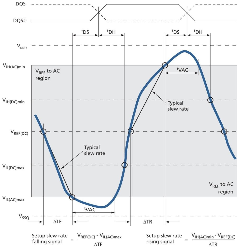
Figure 84: Typical Slew Rate – t<sub>DH</sub> for DQ Relative to Strobe
