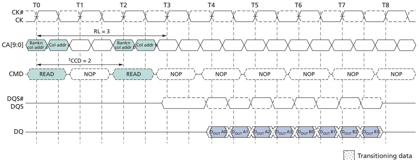
A seamless burst READ operation is supported by enabling a READ command at every other clock cycle for BL = 4 operation, every fourth clock cycle for BL = 8 operation, and every eighth clock cycle for BL = 16 operation. This operation is supported as long as the banks are activated, whether the accesses read the same or different banks.
