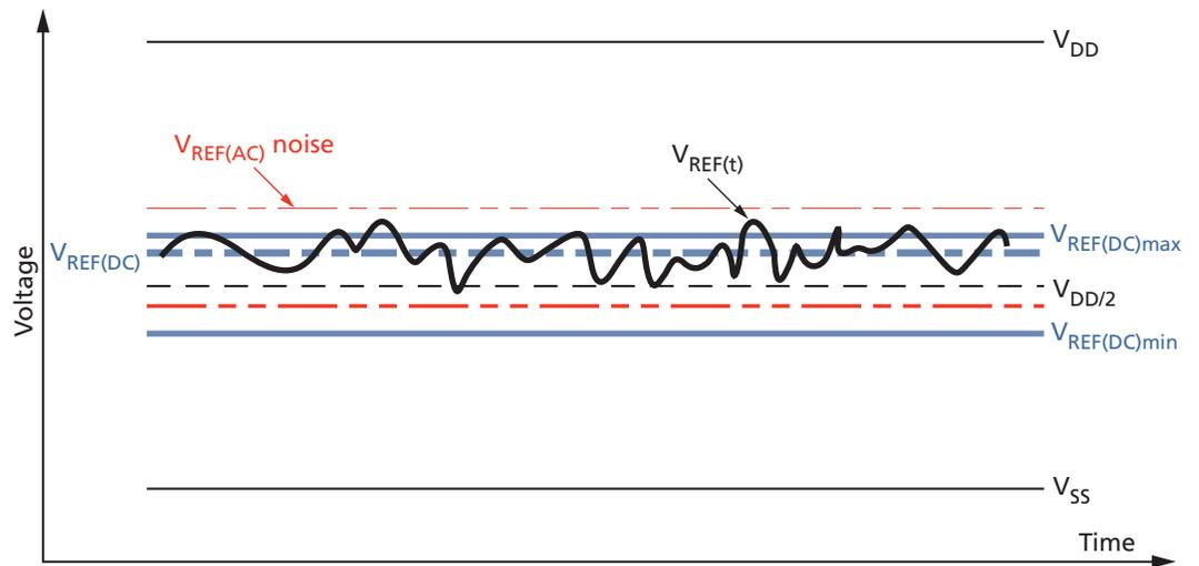
The voltage levels for setup and hold time measurements  $V_{IH(AC)}$ ,  $V_{IH(DC)}$ ,  $V_{IL(AC)}$ , and  $V_{IL(DC)}$  are dependent on  $V_{REF}$ .
