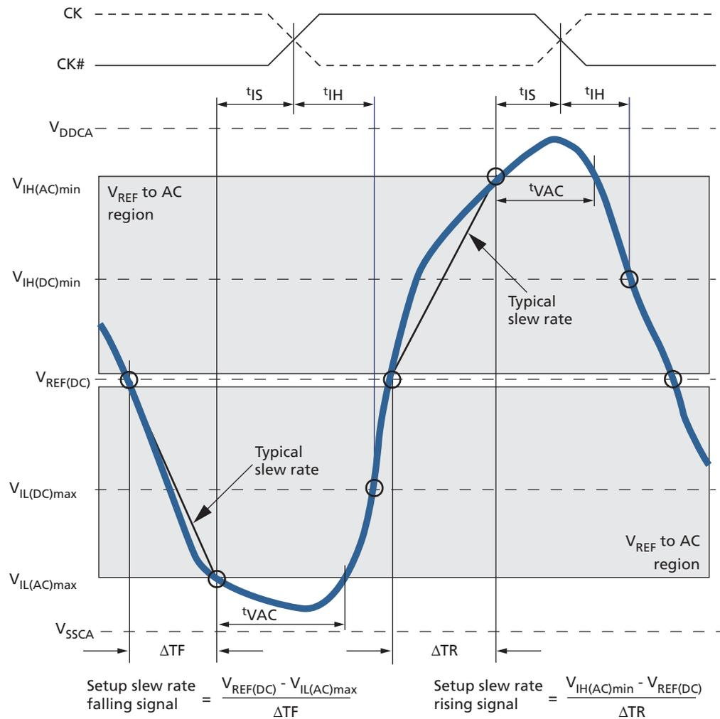
**Figure 80: Typical Slew Rate –  $t_{IH}$  for CA and CS# Relative to Clock**
