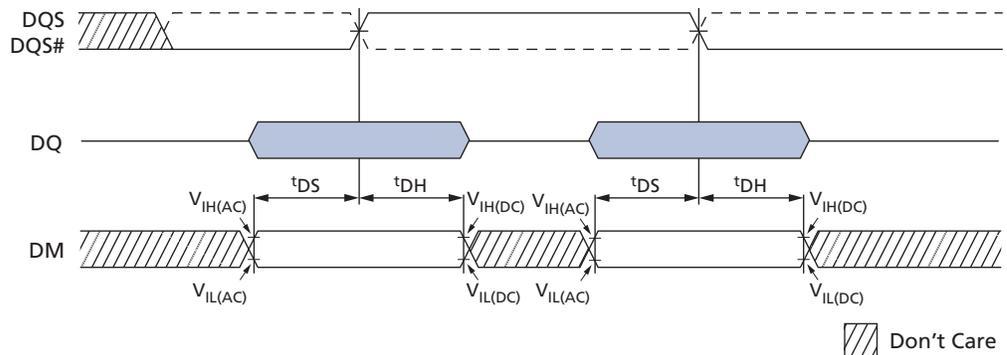
Figure 30: Write Data Mask – Second Data Bit Masked
