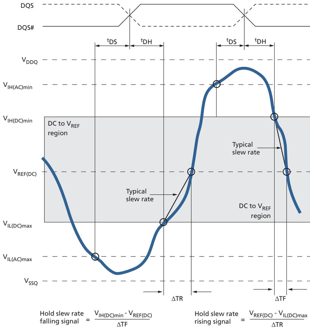
**Figure 85: Tangent Line – t<sub>DS</sub> for DQ with Respect to Strobe**
