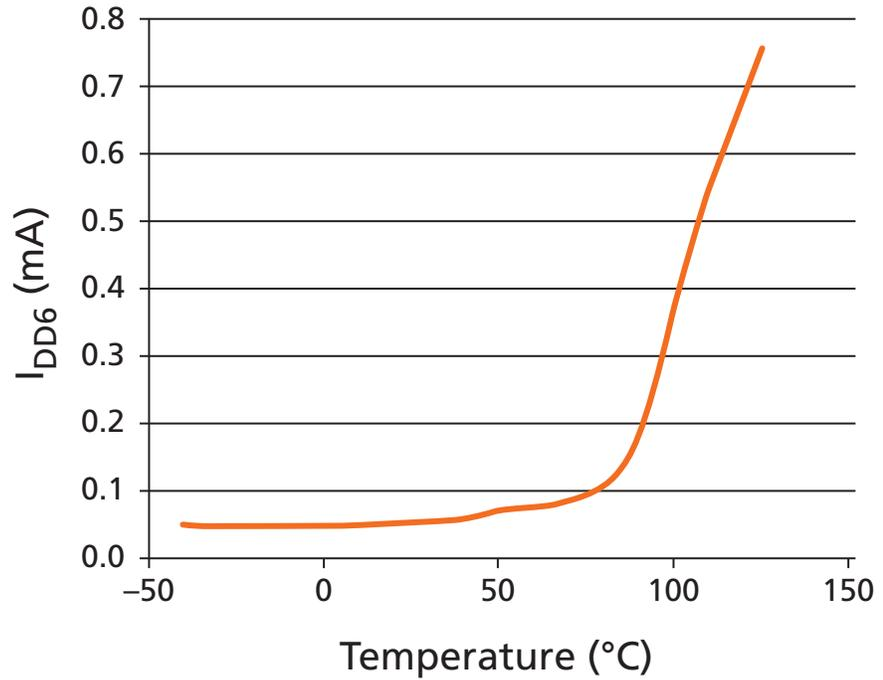
Figure 3:  $V_{DD2}$  Typical Self-Refresh Current vs. Temperature
