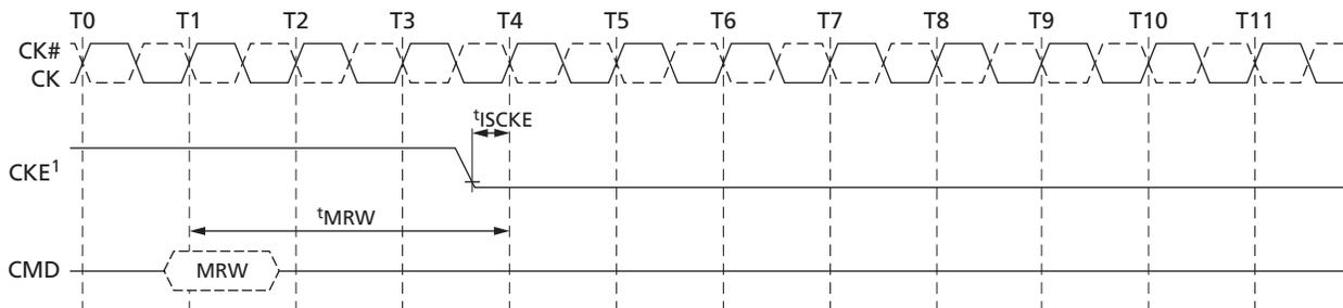
Note: 1. CKE can be registered LOW  $t_{\text{MRW}}$  after the clock on which the MRW command is registered.
