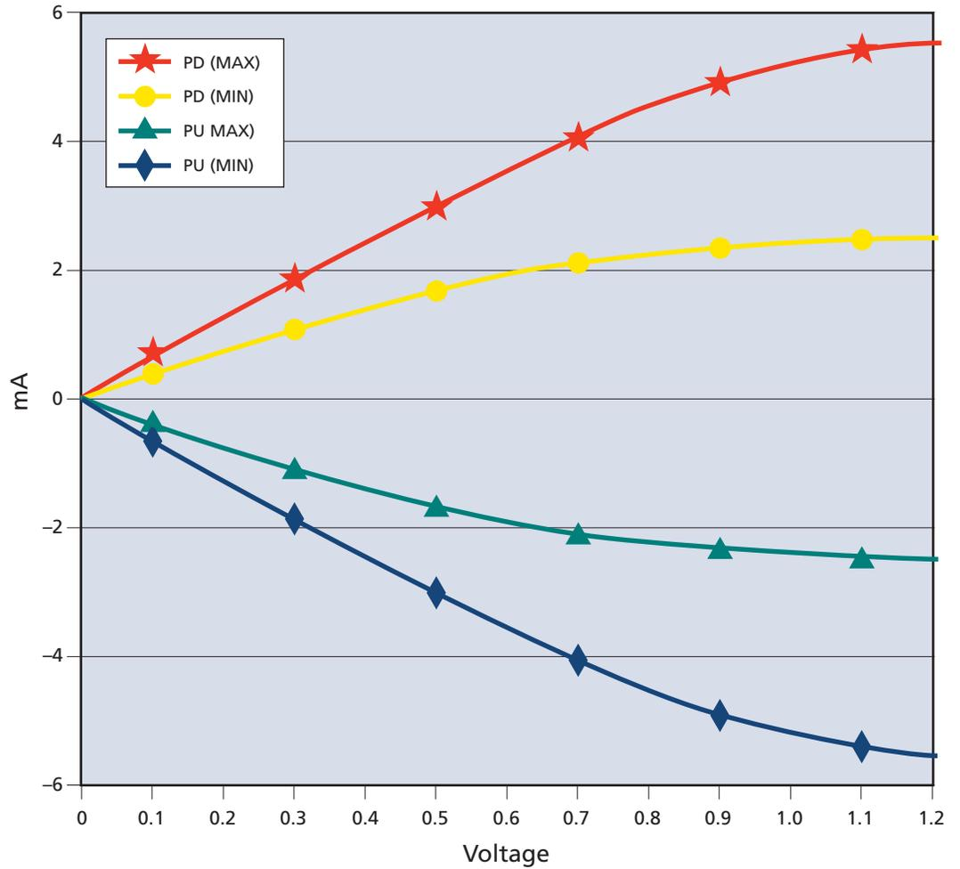
**Figure 77: Output Impedance = 240 Ohms, I-V Curves After Calibration**
