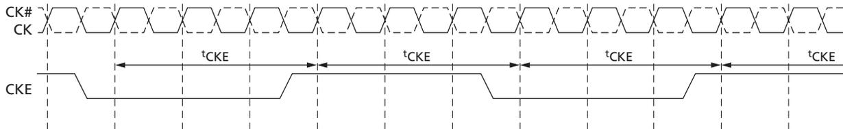
Figure 52: REFRESH-to-REFRESH Timing in CKE Intensive Environments
