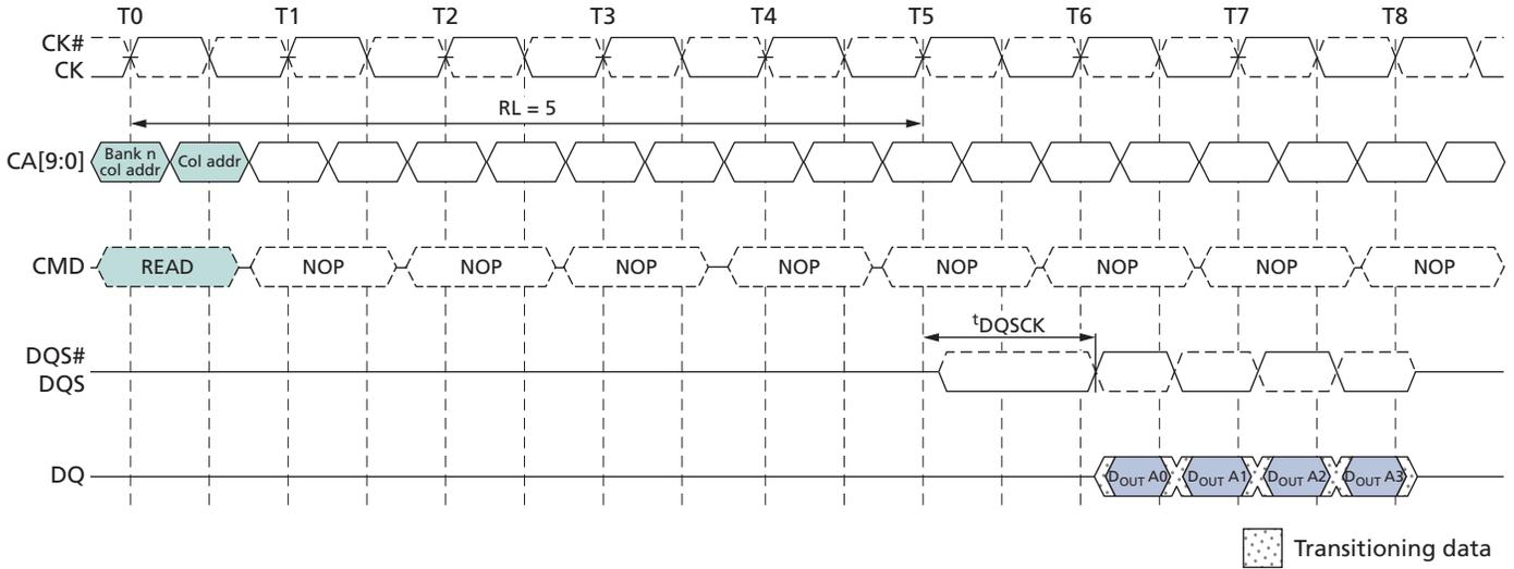
Figure 15: Burst READ – RL = 3, BL = 8,  $t_{DQSCK} < t_{CK}$
