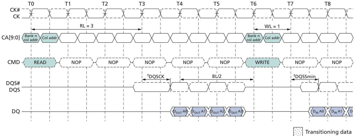
The minimum time from the burst READ command to the burst WRITE command is defined by the read latency (RL) and the burst length (BL). Minimum READ-to-WRITE latency is  $RL + RU(\overset{t}{DQ}SCK(MAX)/\overset{t}{CK}) + BL/2 + 1 - WL$  clock cycles. Note that if a READ burst is truncated with a burst TERMINATE (BST) command, the effective burst length of the truncated READ burst should be used for BL when calculating the minimum READ-to-WRITE delay.
