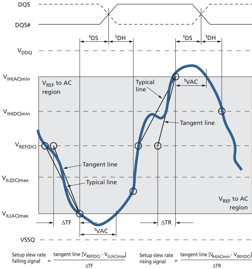
**Figure 86: Tangent Line – t<sub>DH</sub> for DQ with Respect to Strobe**
