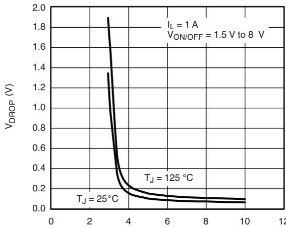
**V<sub>DR</sub>OP vs. V<sub>IN</sub> at I<sub>L</sub> = 1 A**
