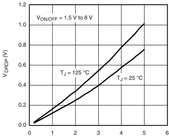
**V<sub>DR</sub>OP vs. I<sub>L</sub> at V<sub>IN</sub> = 4.5 V**
