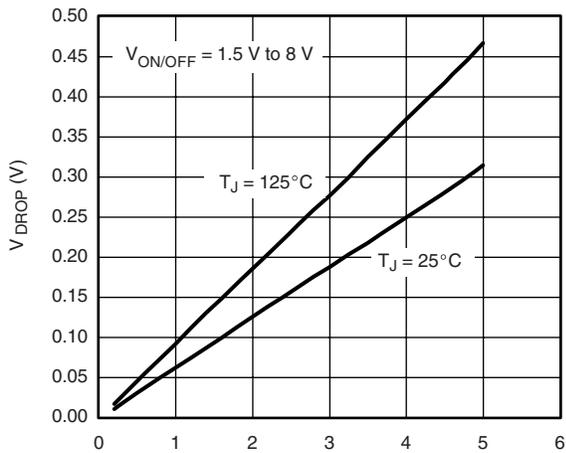
**V<sub>DR</sub>OP vs. I<sub>L</sub> at V<sub>IN</sub> = 10 V**
