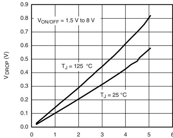
**V<sub>DR</sub>OP vs. I<sub>L</sub> at V<sub>IN</sub> = 5 V**
