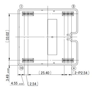
%The dimensional tolerance without directions is  $\pm 0.5$ mm. %Rounded numbers are pin numbers.
