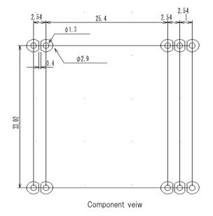
※ 1pin and 2pin are connected by providing land. Mechanical strength may decrease.
