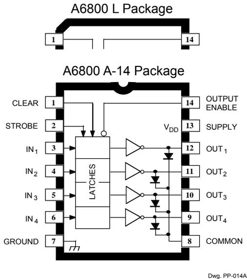
Note: The A6800 SOIC and DIP packages are electrically identical and share a common terminal number assignment.
