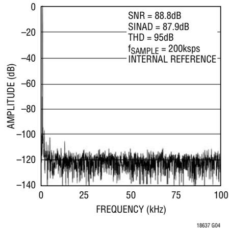
Figure 3. LTC1867 Nonaveraged 4096 Point FFT Plot
