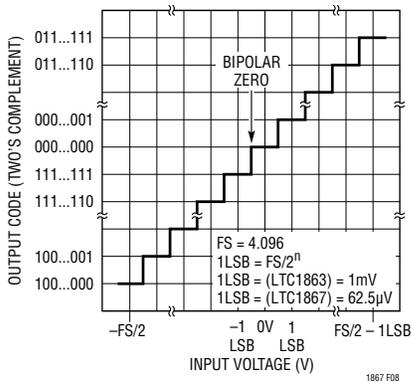
**Figure 8. LTC1863/LTC1867 Bipolar Transfer Characteristics (Two's Complement)**
