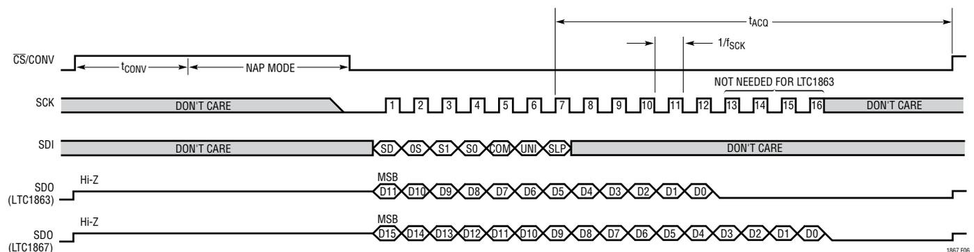
**Figure 6. Example 1,  $\overline{\text{CS/CONV}}$  Starts a Conversion and Remains HIGH Until Next Data Transfer. With  $\overline{\text{CS/CONV}}$  Remaining HIGH After the Conversion, Automatic Nap Modes Provides Power Reduction at Reduced Sample Rate.**
