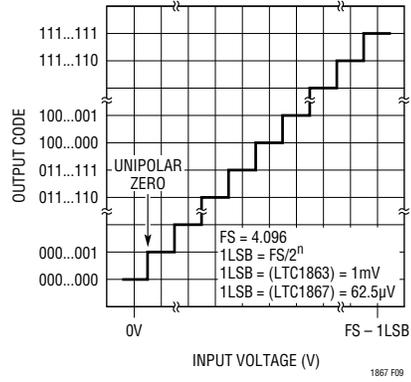
**Figure 9. LTC1863/LTC1867 Unipolar Transfer Characteristics (Straight Binary)**
