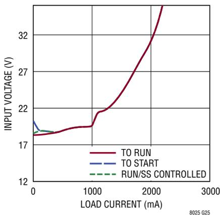
**Minimum Input Voltage vs Load
