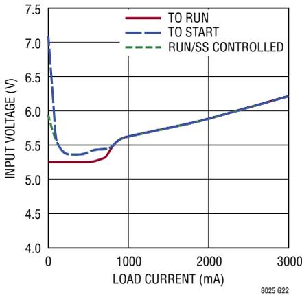
**Minimum Input Voltage vs Load
