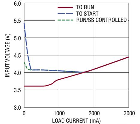
**Minimum Input Voltage vs Load
