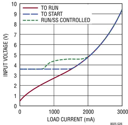
**Minimum Input Voltage vs Load
