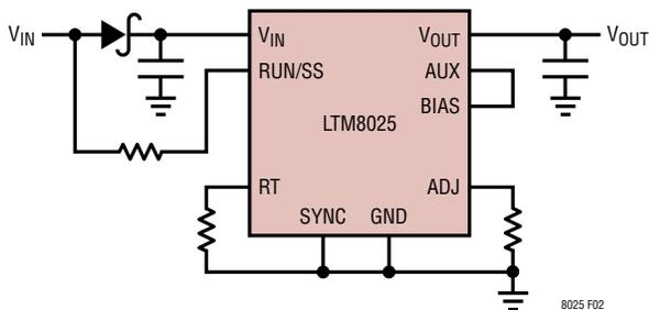
**Figure 2. The Input Diode Prevents a Shorted Input from Discharging a Backup Battery Tied to the Output. It Also Protects the Circuit from a Reversed Input. The LTM8025 Runs Only When the Input is Present.**
