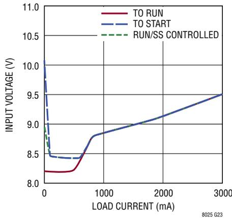
**Minimum Input Voltage vs Load
