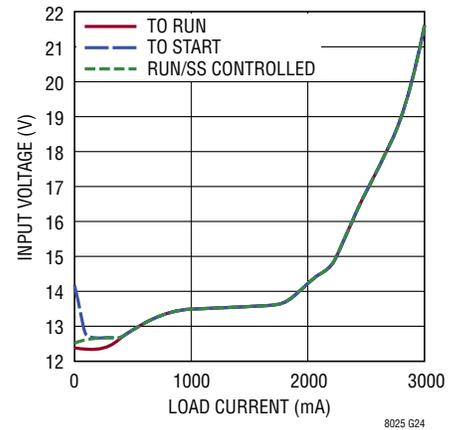
**Minimum Input Voltage vs Load
