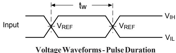
**Voltage Waveforms - Pulse Duration**
