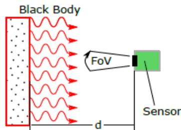
A fluid heated plane black body with an outer dimension covering at least 4 times the sensors field-of-view (FoV) and an emissivity of better than 95% has a surface temperature  $T_{obj}$ . The surface temperature uniformity is better than 0.2°C. The ambient temperature  $T_{amb}$  is at  $25\text{ °C} \pm 3\text{ °C}$ . The TPiS 1T 1086 L5.5 sensor is mounted at a distance d to the black body. Numbers are specified in table 8.
