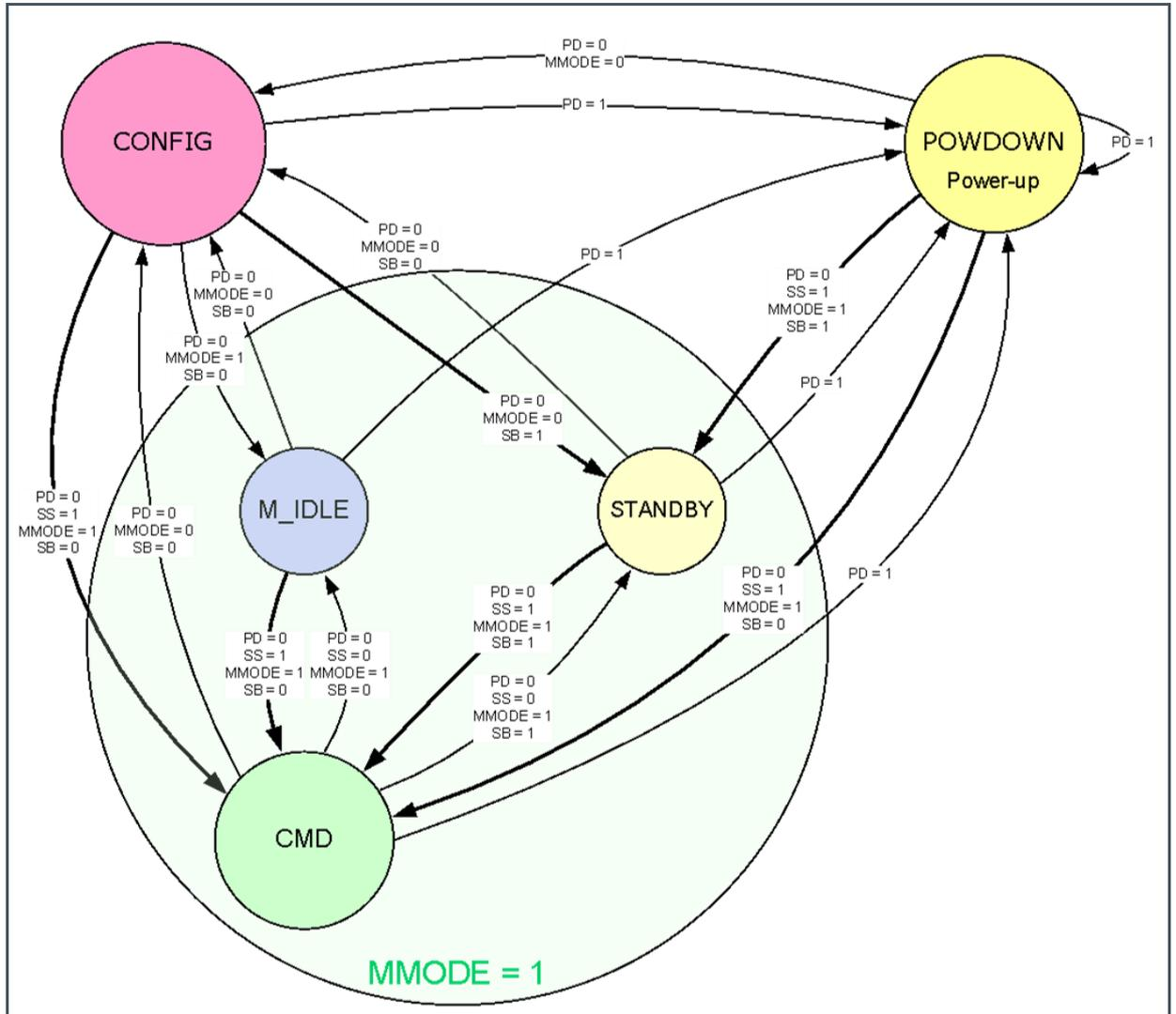
Figure 17 shows the principle sequence for a measurement start in CMD mode coming from Configuration state and waiting in Measurement state between the measurements is shown as IDLE:
