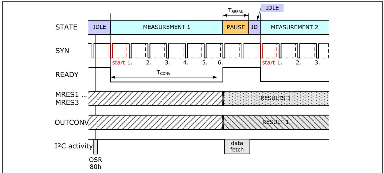
The conversion time ( $T_{CONV}$ ) is determined by the duration between the edges of start and stop of the signal SYN. If  $CREG2:EN\_TM$  is set to '1', the register OUTCONV contains an equivalent amount of  $T_{CONV}$  as counts of the internal clock. With the value of OUTCONV, the measurement results can be calculated more precisely (see chapter "Conversion Time Measurement in SYND Mode").
