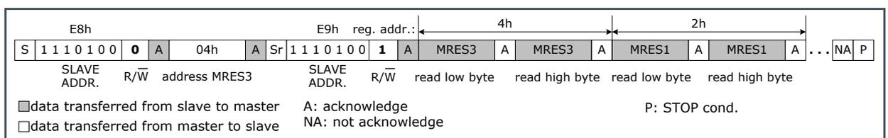
The access of the result register bank with 2 byte each address (starting with the low byte), which is only possible within the Measurement state, has a special feature (see
