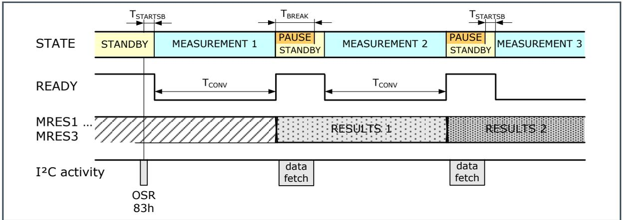
Another example shows, that after the end of a conversion in CMD mode the AS73211 returns to Power Down and/or Standby state depending on the bits OSR:PD and CREG3:SB. In case of both bits are ,0' while in Measurement state the device would return to idle, waiting for the next measurement to start. Figure 24: Principle sequence whereas measurement starts in CMD mode with Power Down and Standby switched on (device is already in Measurement state):
