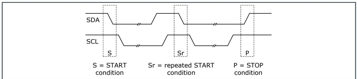
After the protocol started, the data at pin SDA must be stable as long as the high phase of I<sup>2</sup>C clock at pin SCL takes. The change of the communication data at pin SDA is only allowed during the low phase of SCL clock.
