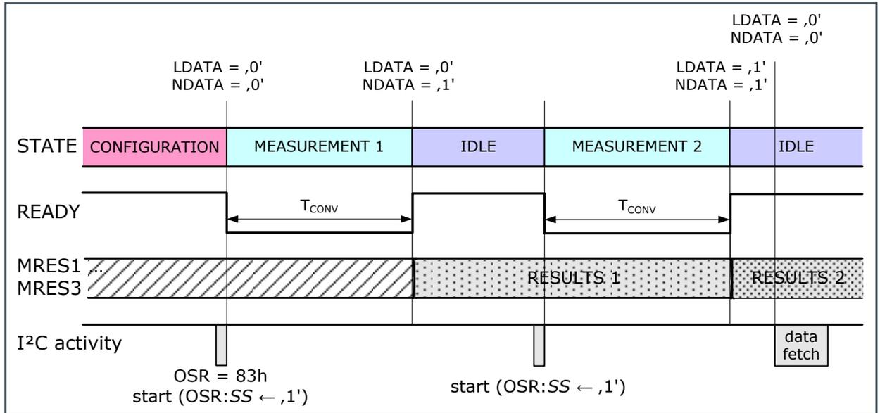
The status bits STATUS:STANDBYSTATE and STATUS:POWERSTATE always show the actual status of the internal control signals for Standby and Power Down. In both cases it can differ from the actual set bits CREG3:SB and OSR:PD, because of the behavior of the control signals while a measurement is in process. The reading of the 16-bit values of the output result registers always starts with the least significant byte.
