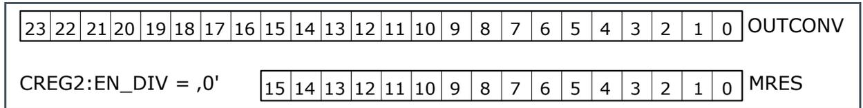
Figure 36 shows the width of the register for the conversion time (OUTCONV), which represents the internal resolution of the A/D conversion. Furthermore the measurement result (MRES[1...3]) is shown, which is 16 bits wide. For all conversion times from  $2^{10}$  to  $2^{16}$  there is no need to use the divider, because OUTCONV is limited to the conversion time length.
