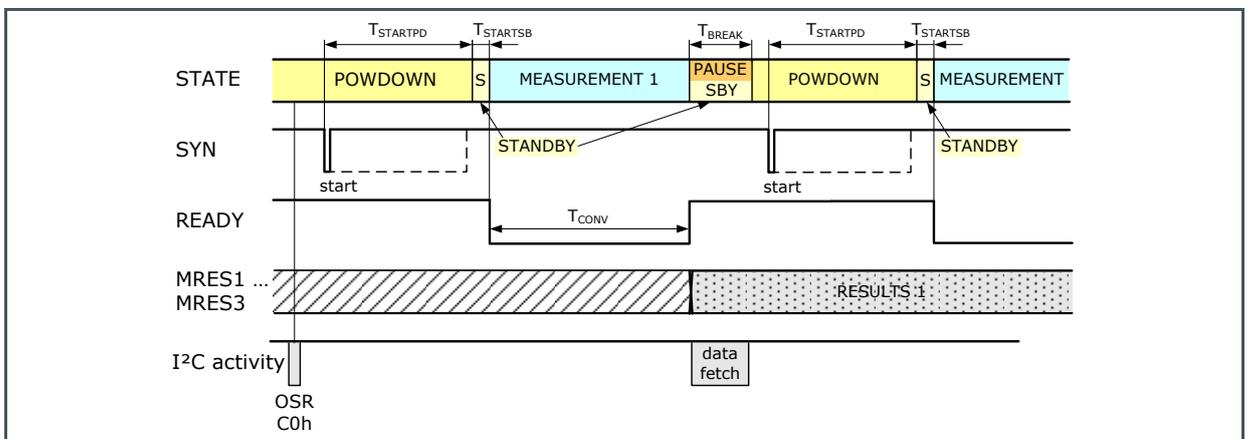
The following example of a SYNS mode shows a correct measurement procedure but with an unfavorable chosen application. After start of measurement with bit OSR:SS = ,1' only the red marked falling edges (see Figure 27) at pin SYN are accepted as start condition, because of the too tight distances of the SYN edges a lot of falling edges are ignored during startup phase (T<sub>STARTPD</sub>), conversion time (T<sub>CONV</sub>) and pause time (T<sub>BREAK</sub>).
