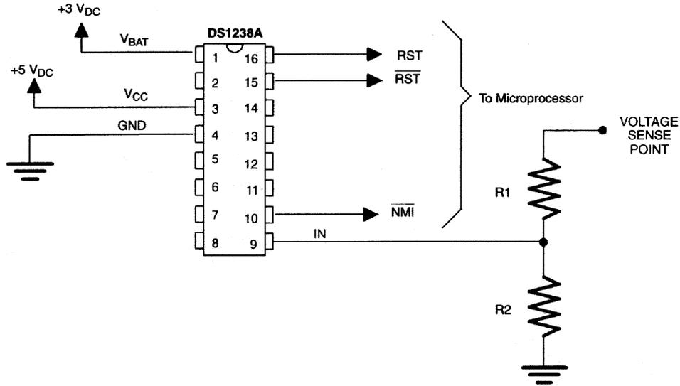
$$V_{\text{SENSE}} = \frac{R1+R2}{R2} \times 1.27$$
