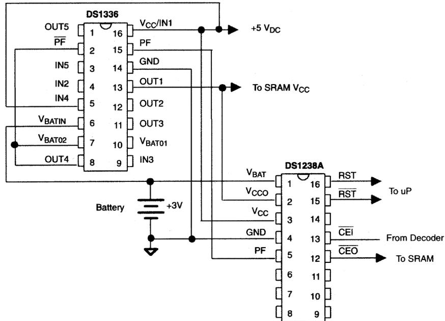
Note: If freshness on the DS1238A is not used,  $\overline{\text{PF}}$  on the DS1336 may be tied to OUT1. This will free IN4, OUT4, and  $V_{\text{BAT01}}$  for system use.
