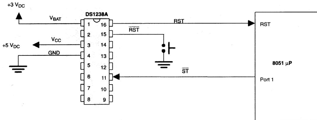
**PUSHBUTTON RESET TIMING Figure 4**
