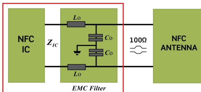
The matching circuit should be designed to match the IC impedance  $Z_{IC}$  to  $100\Omega$  and then connect the antenna through a  $100\Omega$  differential pair.
